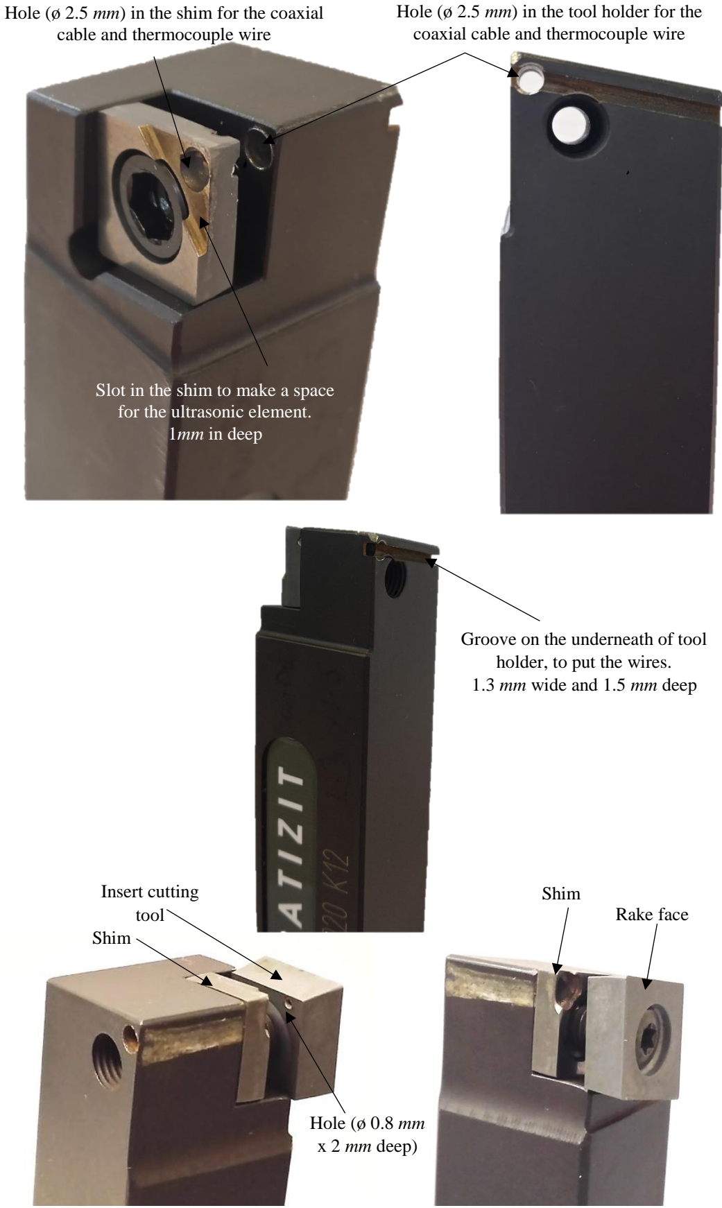
Figure 4.11 Photographs of the modified cutting tool used in this study
