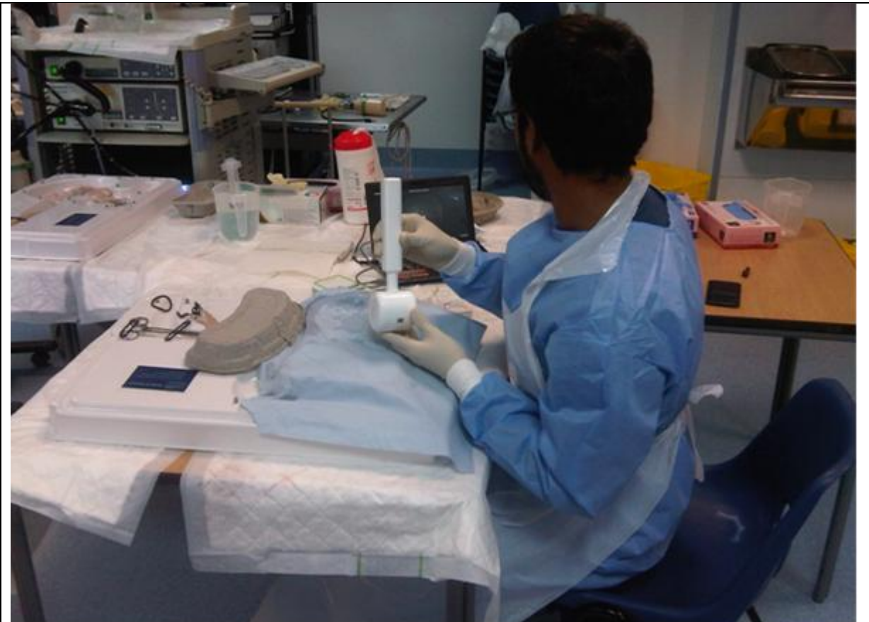
Figure 37: Operator IR performing MACE. The ex vivo porcine stomach tissue is obscured under opaque fabric. The operator is using a rotational movement of the external handheld magnet in a fixed position to give panning views of the gastric cavity, observed on the lap-top computer in real time.
