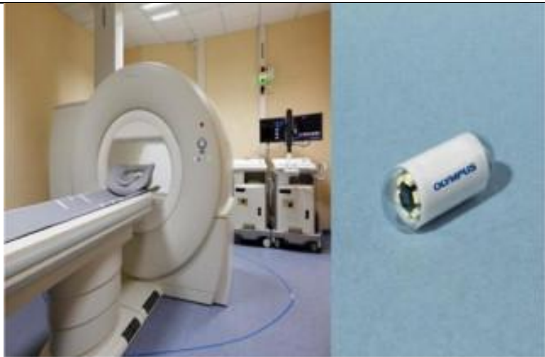
Figure 25: The Olympus and Siemens navigation system, control panel and capsule used by Rey et al. With permission.(199)
