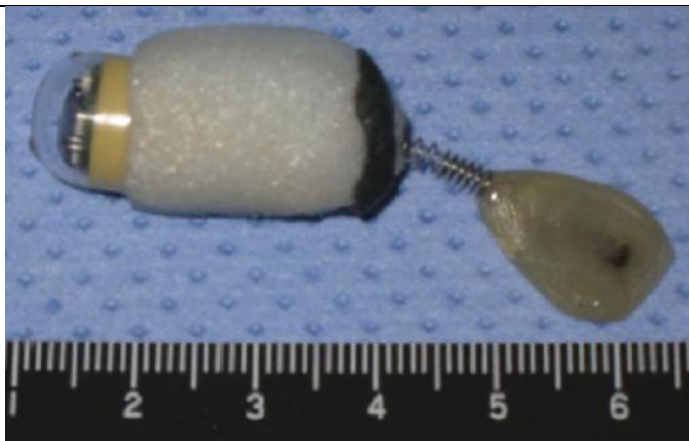
Figure 23: An applied alternating current magnetic field causes vibration of the fin attached to the capsule developed by Morita et al. With permission.(175)
