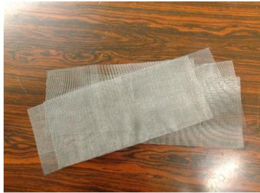
**Figure 3. 20** The photograph of rectangular cuts of the stainless steel screen of the regenerator
