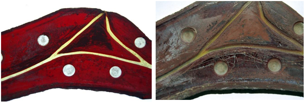
Fig. 50, Fairford, Example of both drilling and hand abrading in transmitted and reflected light.
