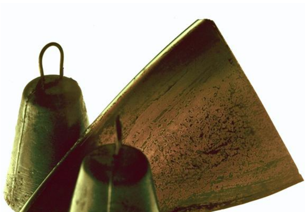
Fig. 32, St. Mary's Fairford. Rounded edge of a spun sheet used uncut for tracery eyelet pieces.
