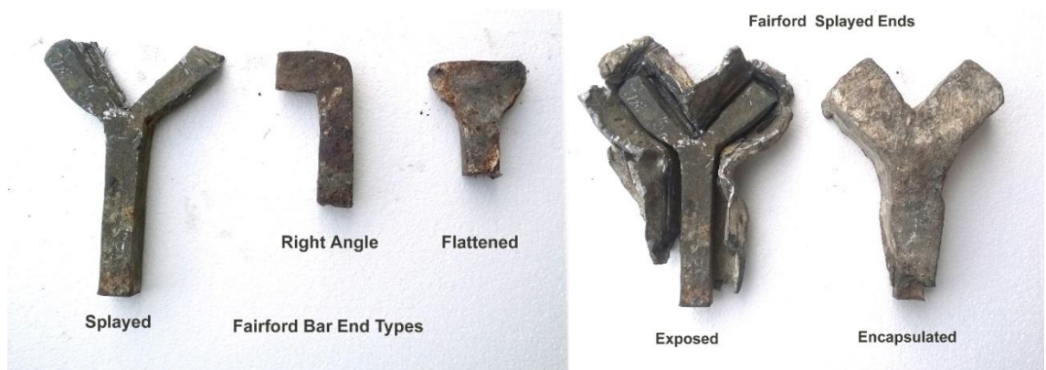
Fig. 6, Fairford, details of three types of ferramenta anchor ends with cast lead coverings.
