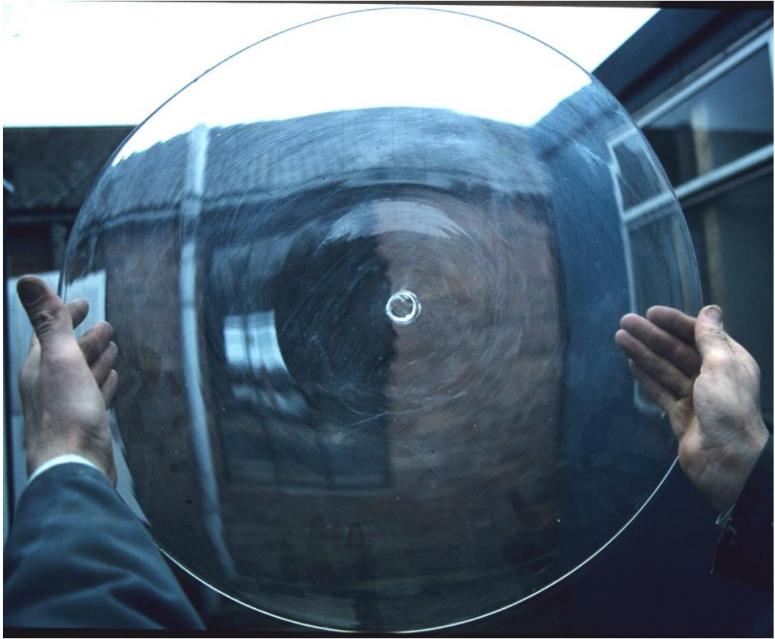
Fig. 33, Modern example of a full sheet of glass produced by the spun process.
