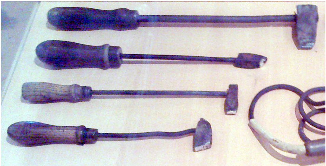
Fig. 72, Examples of soldering irons. Romont, The Swiss Museum of Stained Glass and Glass.
