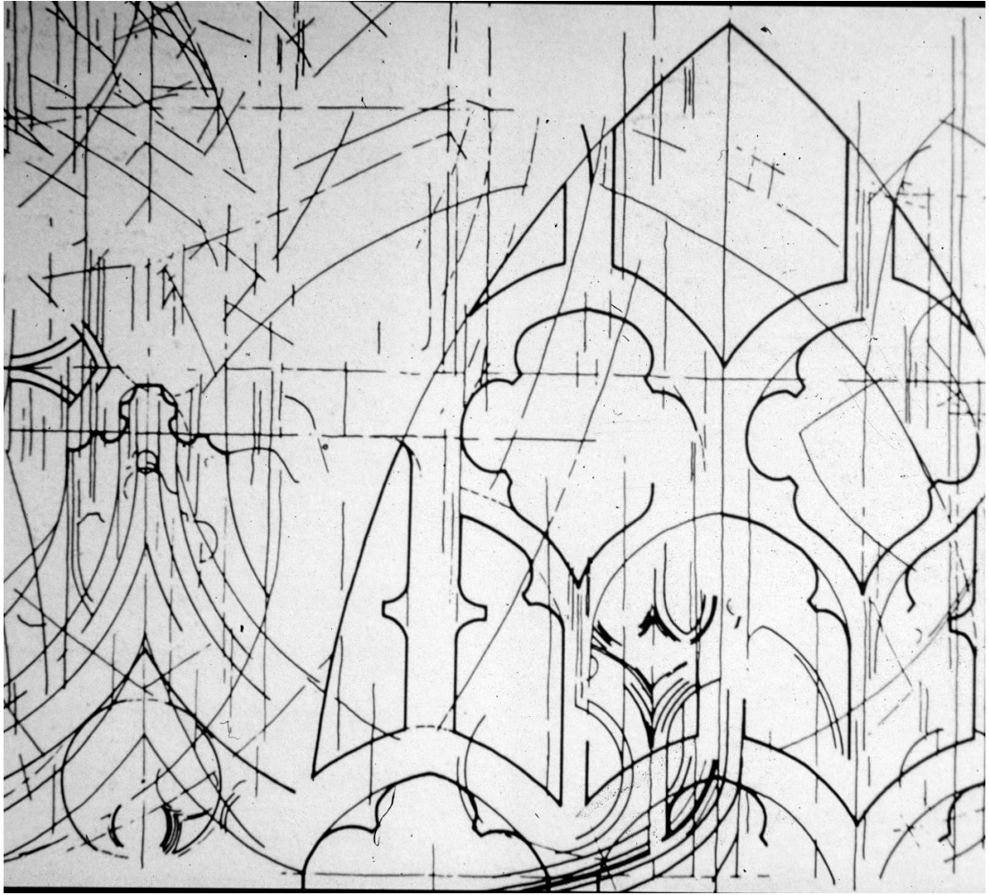
Fig. 15, York Minster, example of the geometric setting out for a window tracery.
