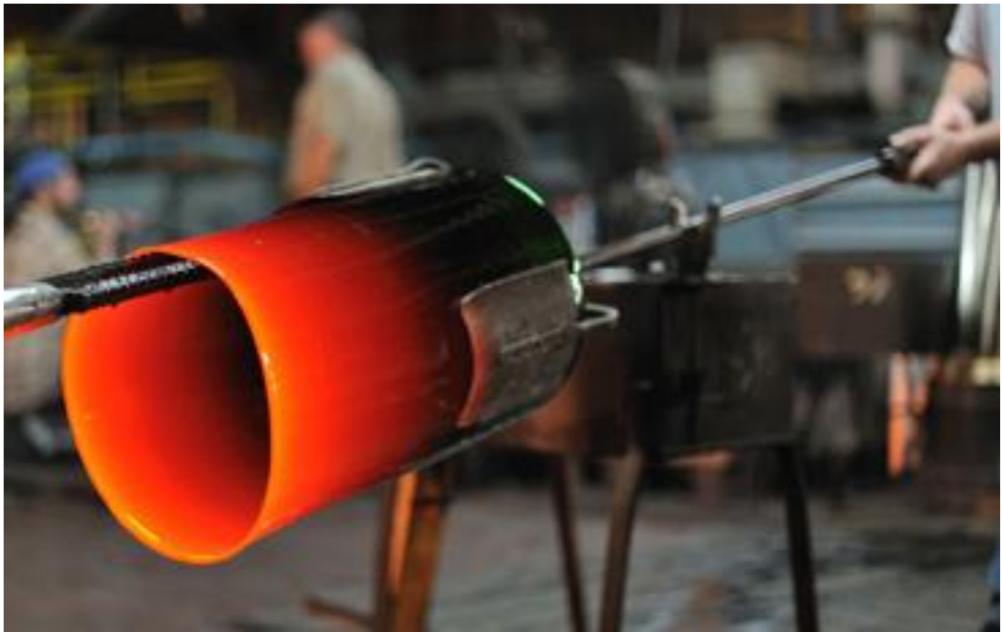
Fig. 29, Cylinder glass in production at Glashütte Lamberts, Waldsassen.
