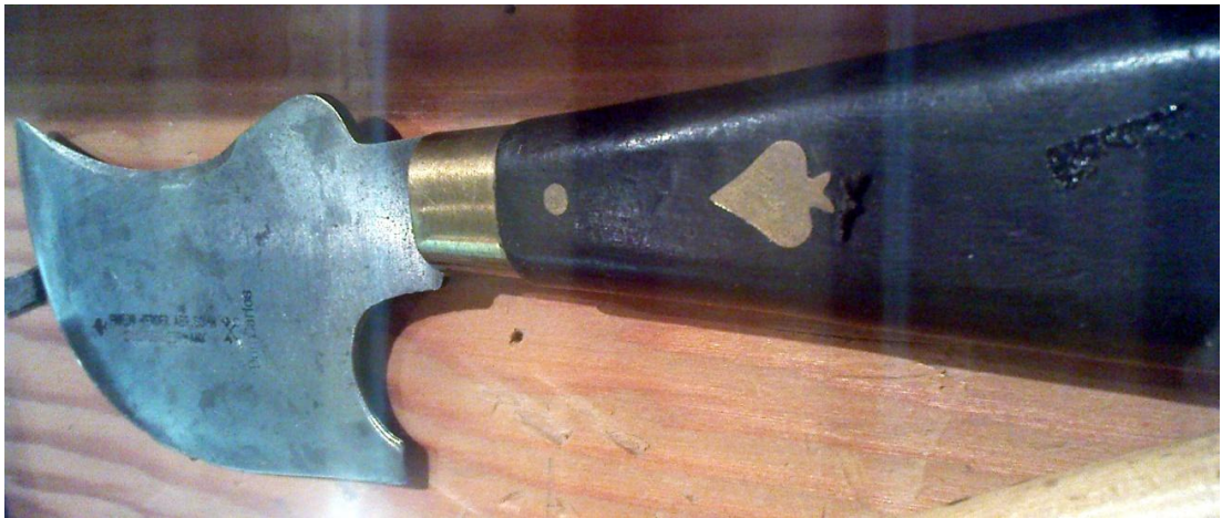
Fig. 71, Example of a curved cutting knife. Romont, The Swiss Museum of Stained Glass and Glass.
