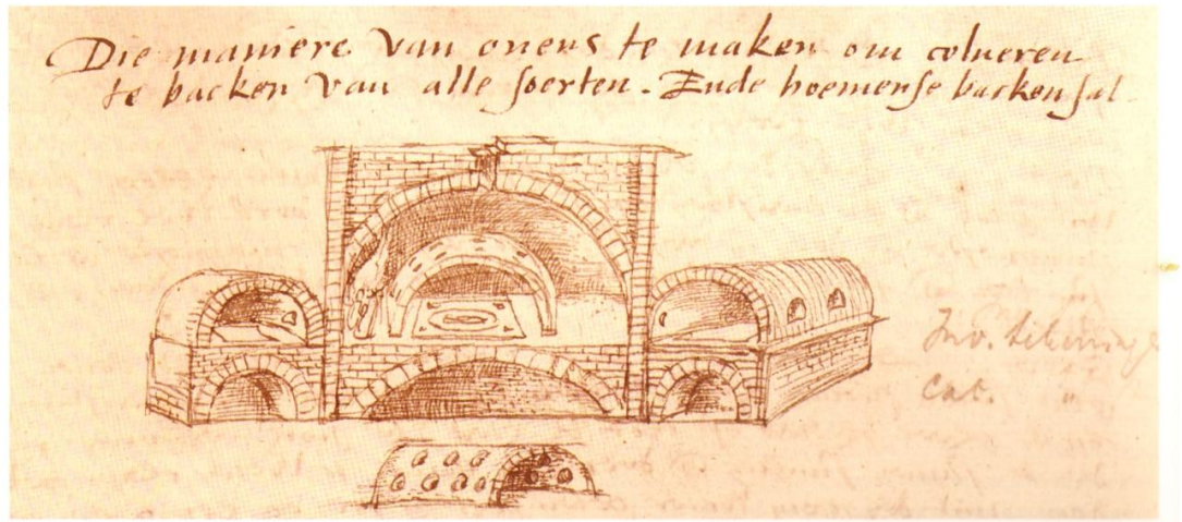
Fig. 66, Three chambered kiln from 16 th century manuscript. Museum Plantin-Moretus, Antwerp, MS no. 64 f° 33.
