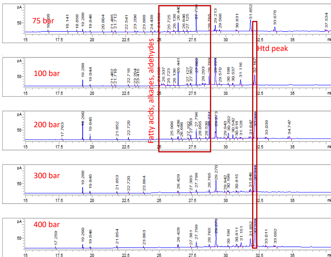
Figure 3-7: GC-FIDs chromatogram of the fractions from the sequential scCO 2 extraction using 1 g wax: 200 g silica adsorbent at 313 K and 40 min
