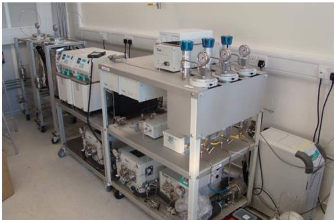
Figure 6-3: The scCO_2 extractor used in the fractionation of the wax
