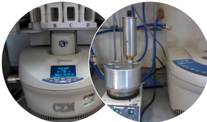
Figure 6-4: Traditional stirrer hot plate and SP discoverer microwave (CEM) heating sources used for the modification of the Htd
