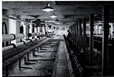
Plate 55 Typical arrangement of spinning mules along the length of a multi-storeyed mill at Quarry Bank Mill, Wilmslow
