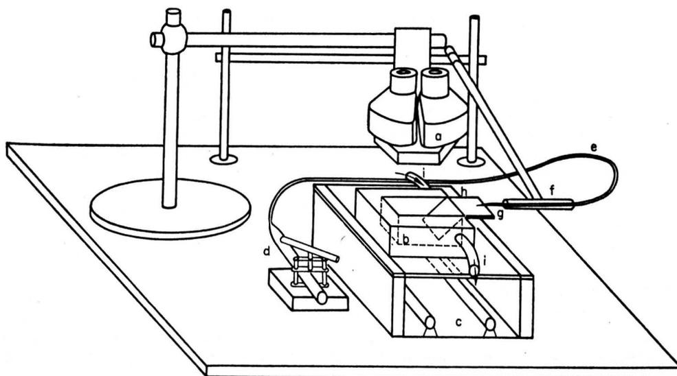
FIG. 1. Diagram of apparatus. Key: a, microscope; b, worm bath; c, fluorescent tubes; d, oil reservoir and screw clamp; e, fine polythene tube; f, guide for polythene tube; g, micropipette; h, Perspex and cork shelf; i, water inlet and outlet.
