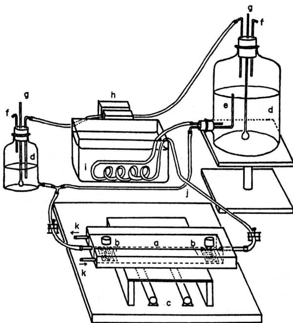
FIG. 1. Diagram of apparatus. Key: a, Perspex worm bath at 37°C; b, cork pieces to which worm pinned; c, fluorescent tubes; d, reservoir of Hank's saline; e, overflow to maintain constant level; f, gas outlet; g, bubbler for gas mixture; h, peristaltic pump to return saline from small to large reservoir; i, glass coil in water bath to warm saline to 37°C; j, polythene tubing to conduct saline; k, inlet and outlet to water jacket at 37°C.
