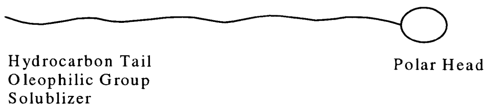
Figure 1.2. A typical additive with a polar end group and a hydrocarbon tail.
