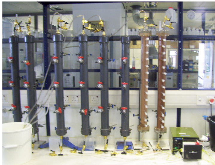
Figure 4-3: Picture of the new (left) and old style (right) columns in the vertical position.
