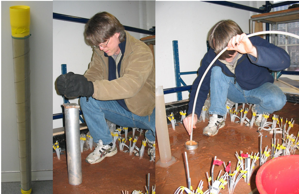
Figure 11-8: Pictures left to right of: New well screen with stainless steel mesh attached, aluminium tube being inserted, sand being slurried out from centre of tube.
