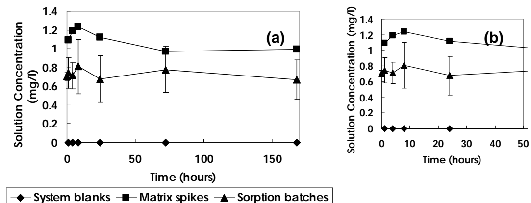
Figure 6-2: Distribution and temporal history of a 1 mg/l addition of TCFE into Permo-Triassic sand with 0.1% activated charcoal (sorption batches). System blanks have no TCFE added and matrix spikes (controls) have no sand or charcoal added. (a) whole experiment, (b) shows detail of early behaviour.
