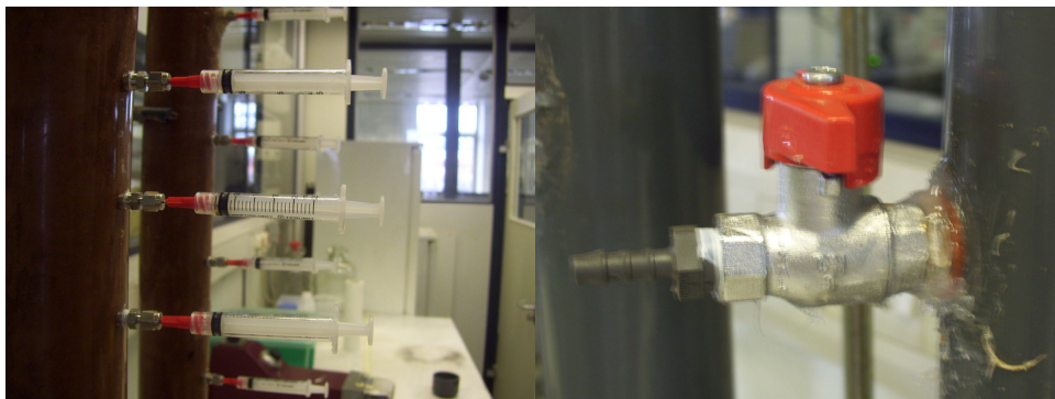
Figure 4-2: Sample ports for the acrylic columns in the left picture and uPVC column in the right picture.
