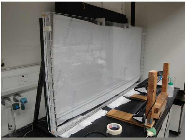
Figure 9-1: Imaging box before well screen insertion and bead packing
