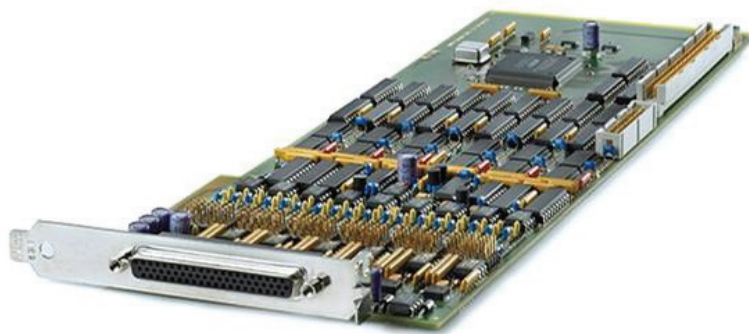
Fig. 2.37. DS3001 incremental encoder interface board [DSP10].
