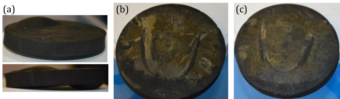
Figure 6-10: Digital Photographs of (a) BA40, (b) BA50 and (c) BA60 Following 250 kGy Gamma Radiation under 3.2 MPa CO 2
