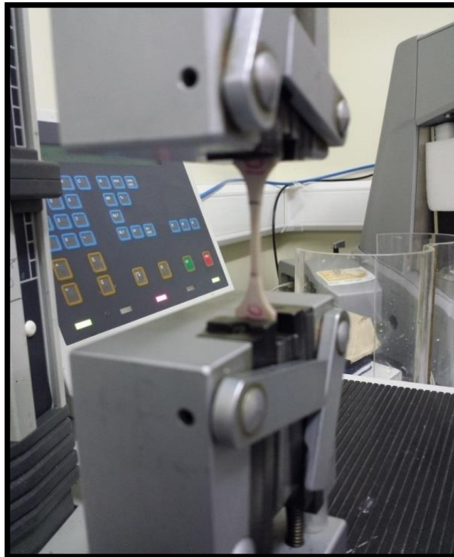
Figure (7-21): PEEK specimen undergoing tensile testing procedure
