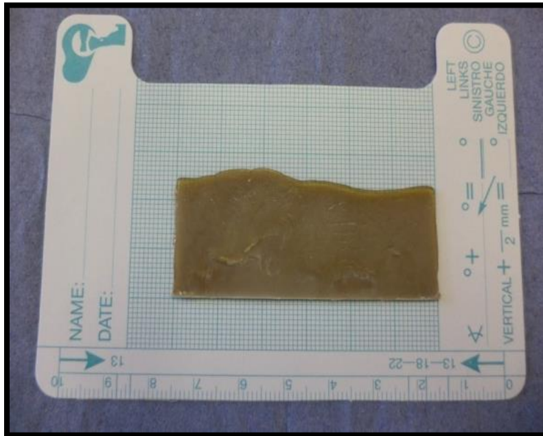
Figure (3-4): PEEK specimen flow measured mechanically using graph paper
