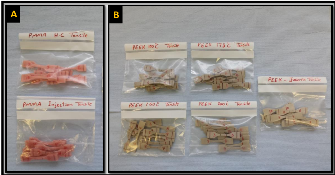
Figure (7-20): Tensile sample ready for testing. A. Conventional PMMA processed by heat-cured and thermo-pressing techniques; B. PEEK experimental samples fabricated using thermo-pressing technique and CAM production method
