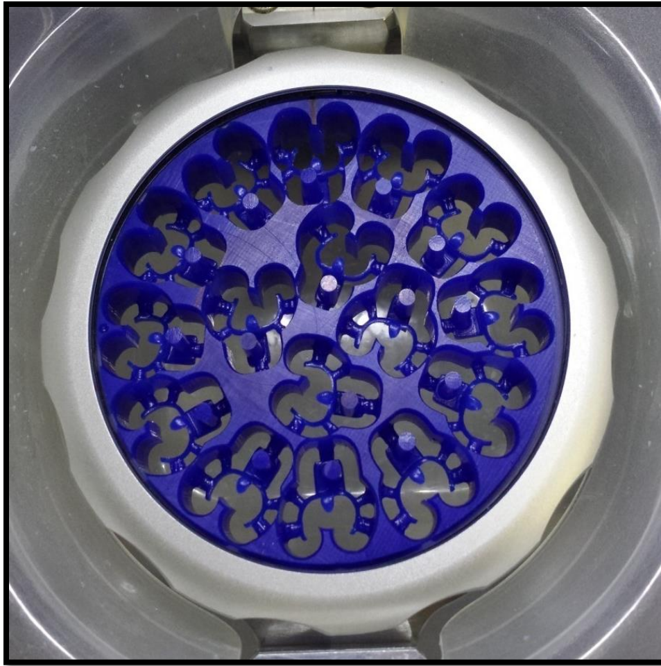
Figure (8-26): Co-Cr wax clasps prepared using milling machine
