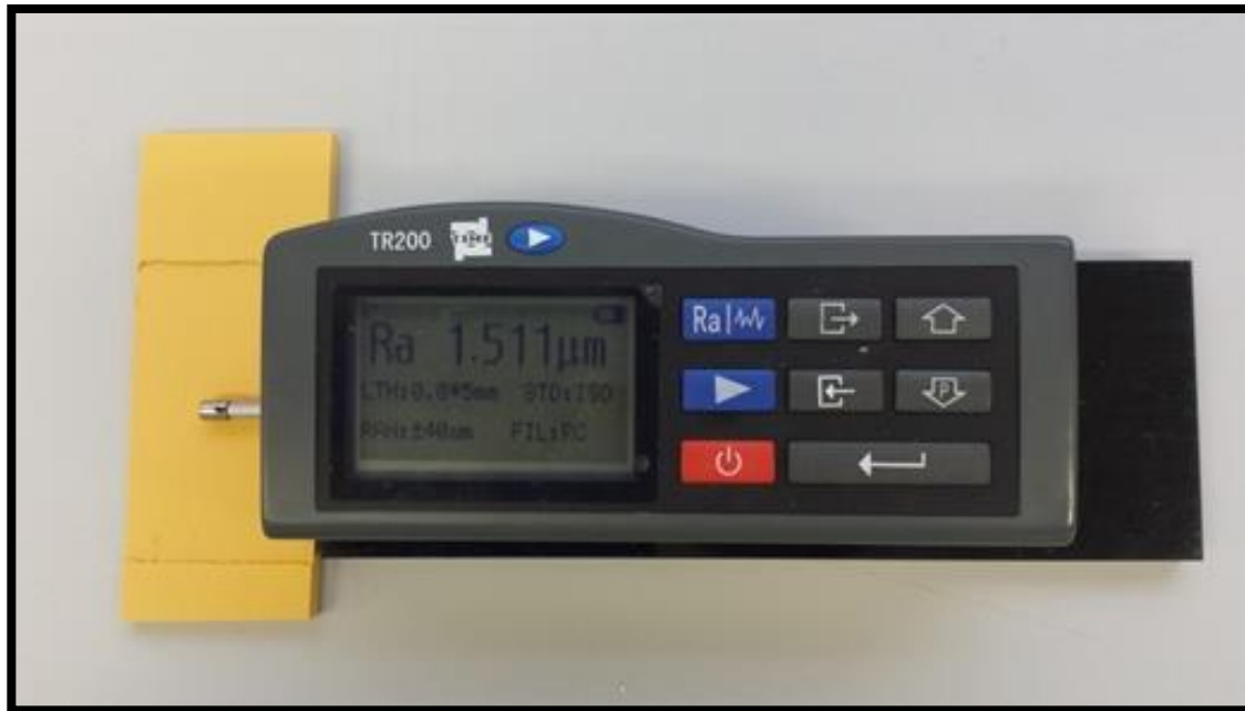
Figure (6-2): Measuring diestone type IV specimen by profilometer surface roughness testing machine
