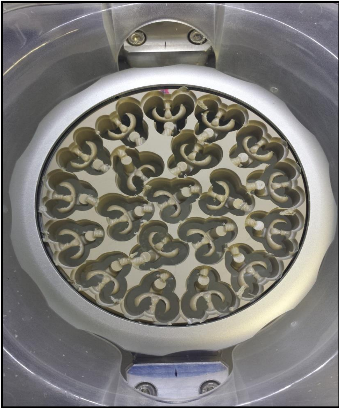
Figure (8-21): PEEK clasps prepared using PEEK-Juvora™ discs
