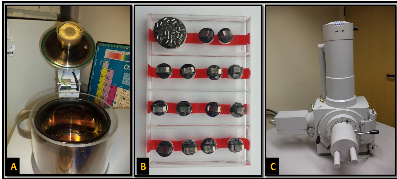
Figure (7-5): A. sputtering device for gold coating; B. specimen prepared with gold coating for SEM; and C. electron optical column unit
