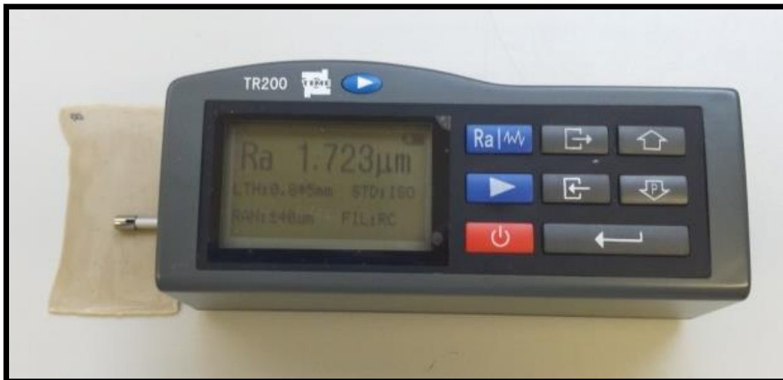
Figure (6-3): Measuring PEEK specimen surface by profilometer surface roughness testing machine
