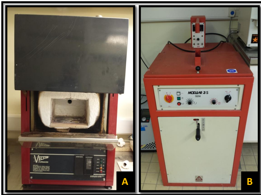
Figure (3-17): A. Vecstar furnace used to preheat the casting ring and to burnout the wax pattern; B. Electronic induction metal casting machine used to cast the metal alloy
