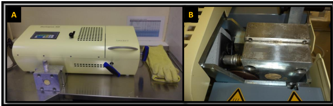
Figure (3-8): A. Thermopress 400 machine used to inject metal-free denture base materials; B. The flask was ejected from the heated chamber after injection of the material into the mould cavity
