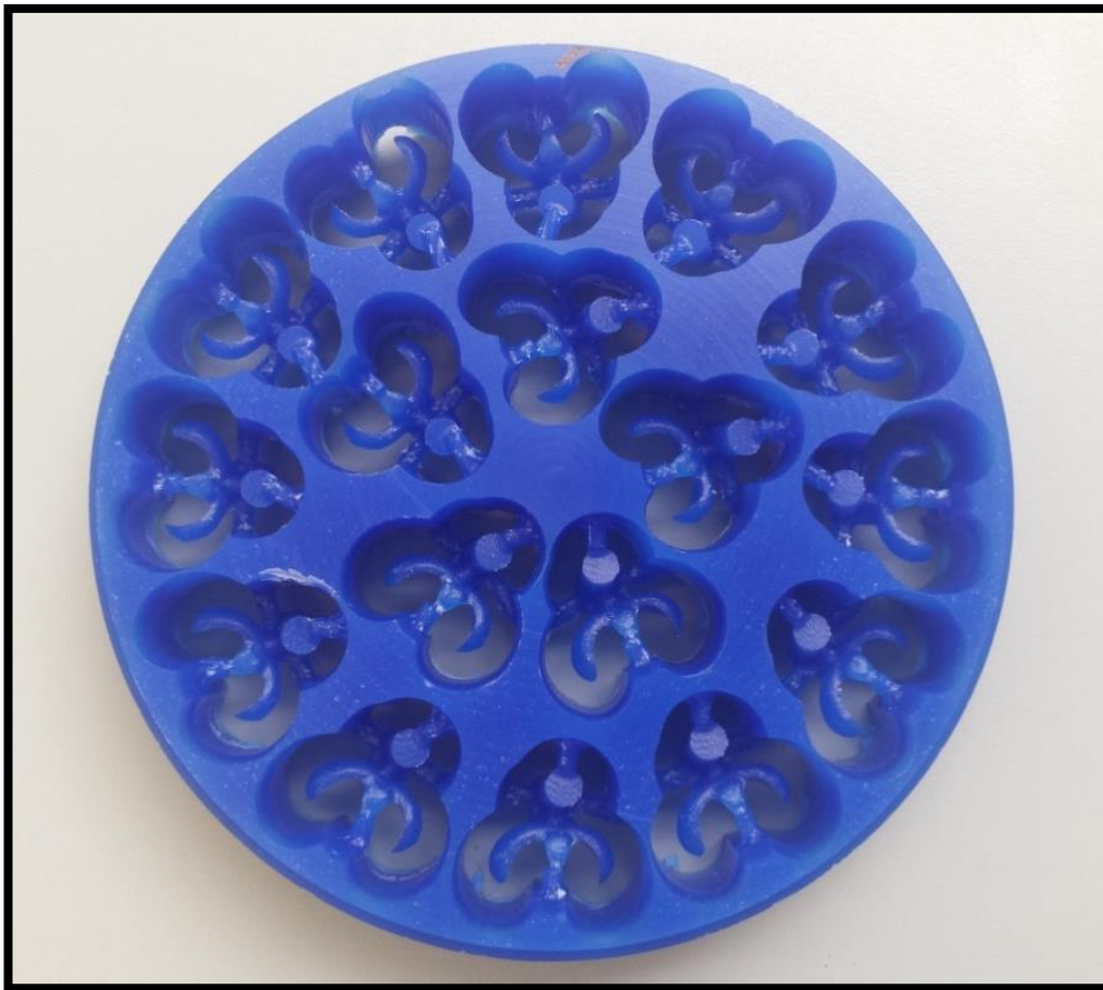
Figure (8-23): Wax clasps prepared using wax discs for thermo-press purposes
