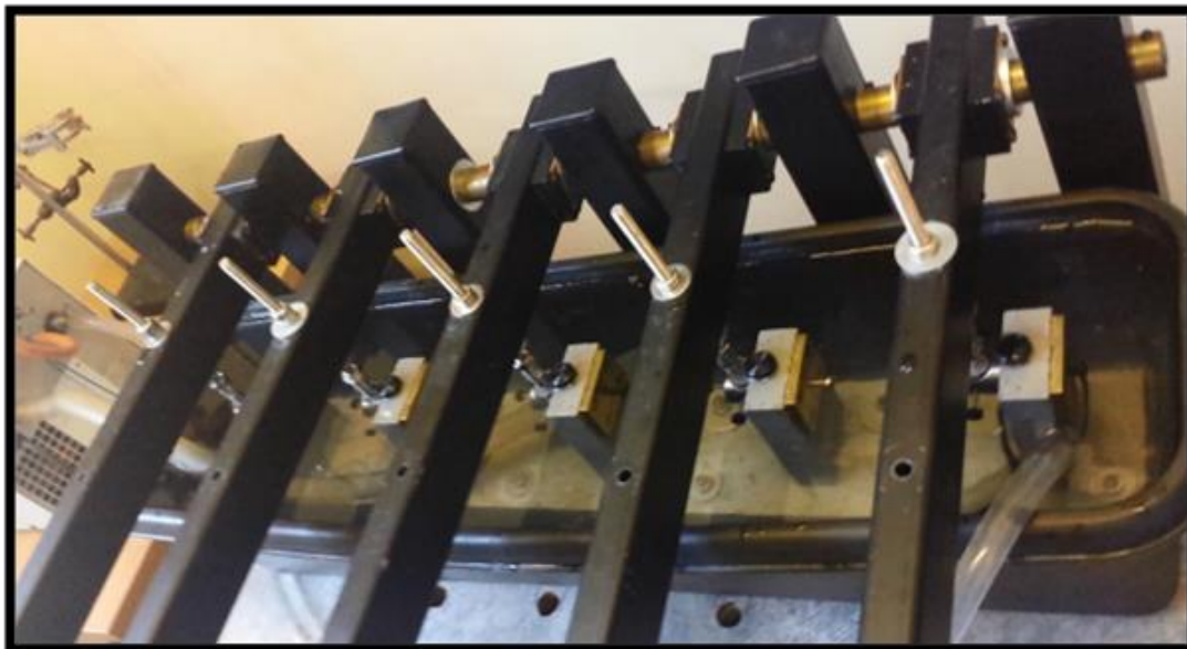
Figure (8-31): Five clasp specimens mounted inside the thermo-cycling water bath tank of the chewing simulator machine
