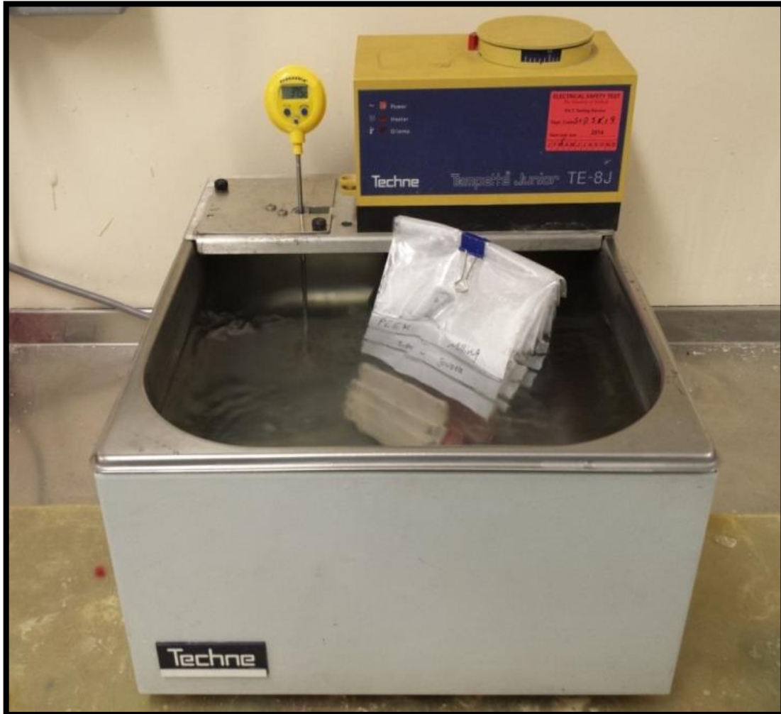
Figure (7-12): Storage of the sample in water for 50 ( \pm 2 h) at 37 ( \pm 1 °C) before the testing procedure
