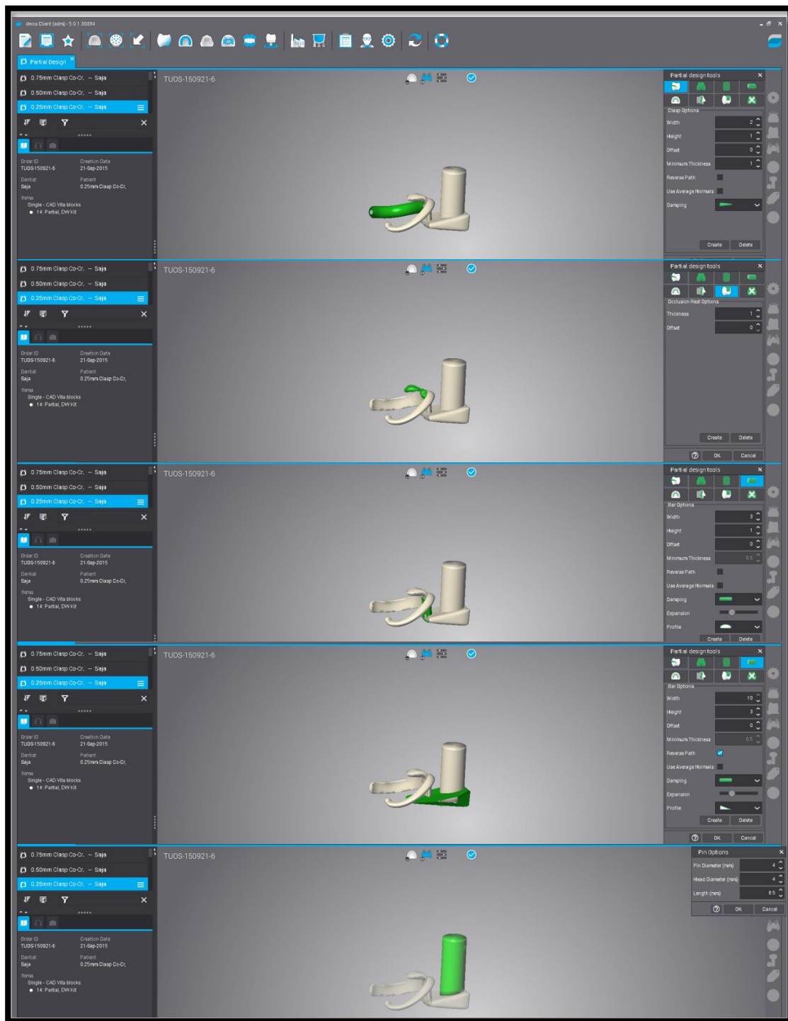
Figure (8-7): Co-Cr clasp design at 0.25 mm undercut with a 2 mm thickness reciprocal arm, occlusal rest, and pin holder for test purposes
