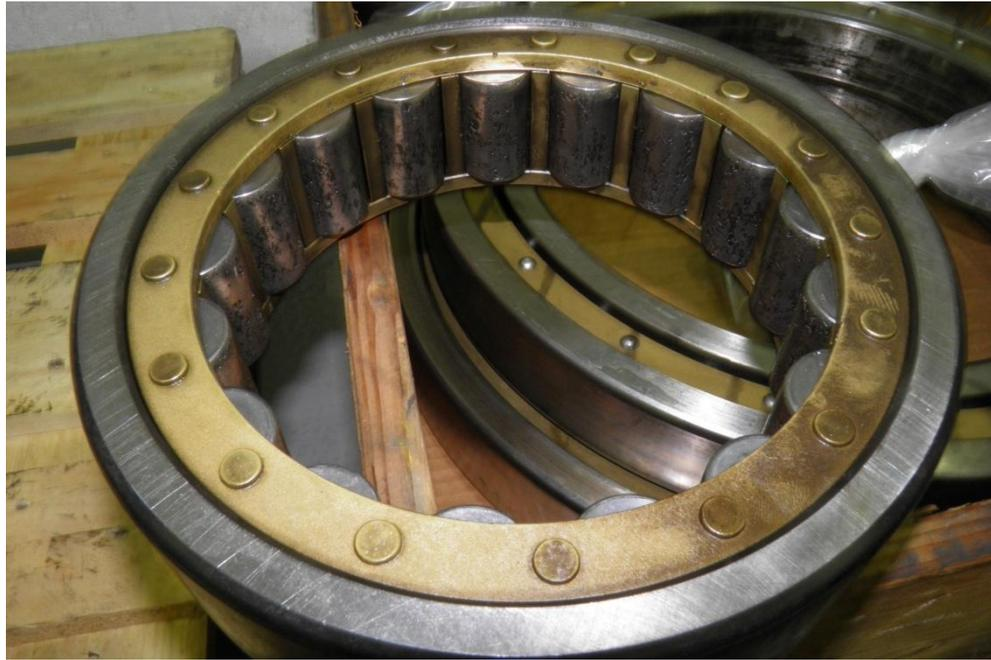
Figure 9-12: Outer race, cage and rolling elements of failed planetary gear bearing
