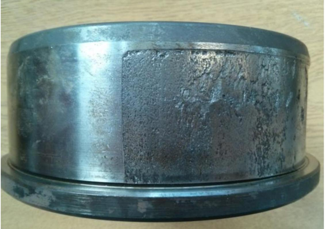
**Figure 9-8: Image showing surface damage and clear transition from undamaged to damaged region**
