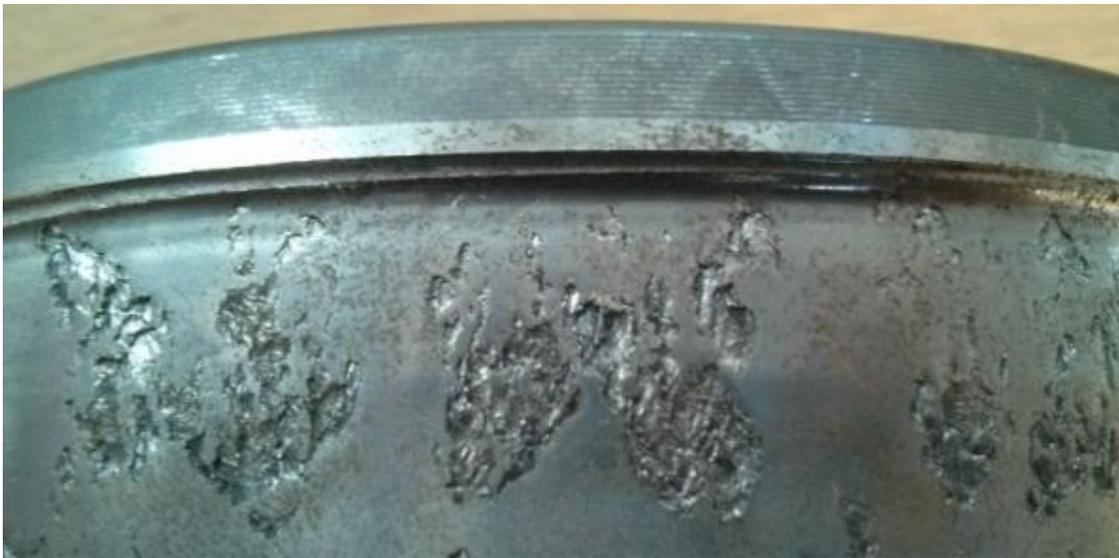
Figure 5-2: Spalling on the raceway surface in Zone 2
