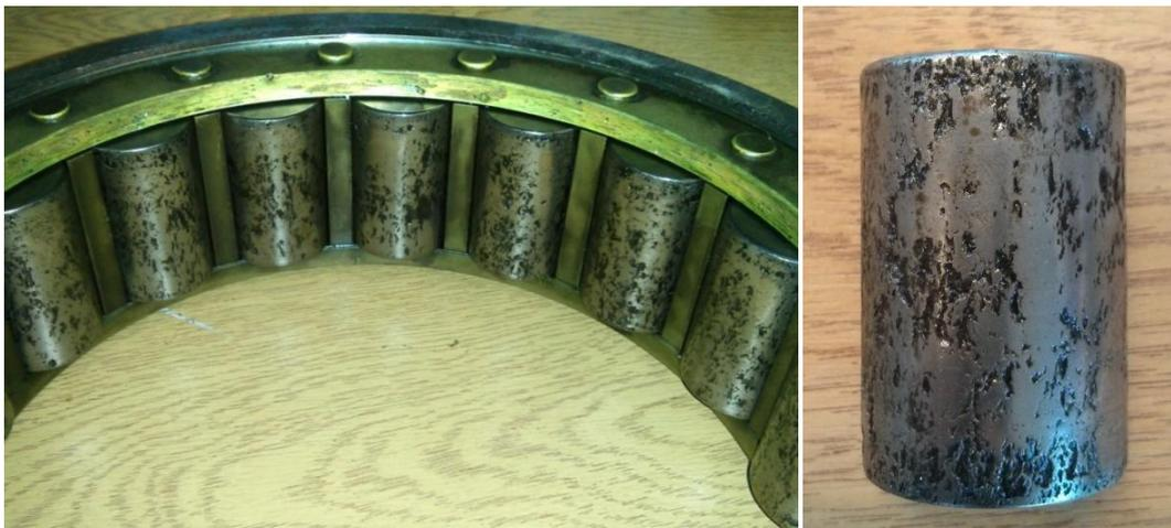
Figure 9-13: Wear scars observed on cylindrical rollers
