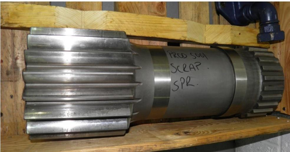
Figure 9-16: Low speed intermediate shaft
