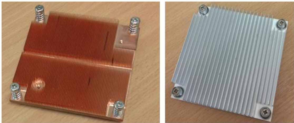
Figure 5-5 The copper heat sink (left) and ‘reduce cost’ aluminum heat sink (right)
