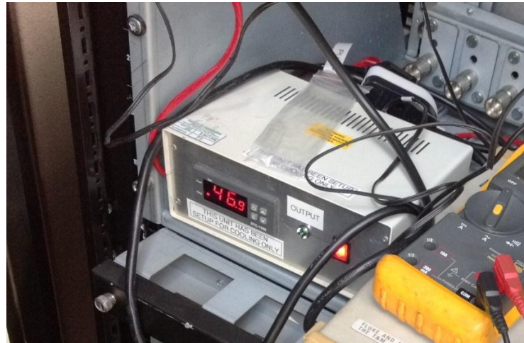
Figure 6-13 Installation and functioning of STC-1000 temperature controller
