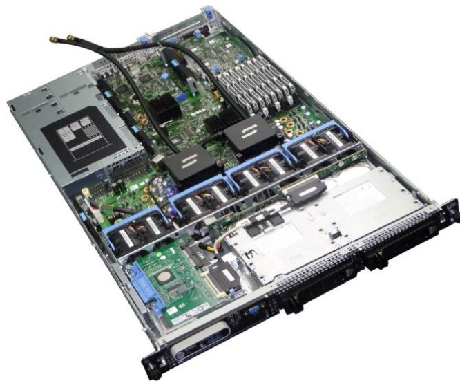
Figure 2-23 CoolIT server blade with water-block cooling design (CoolIT system, 2015).
