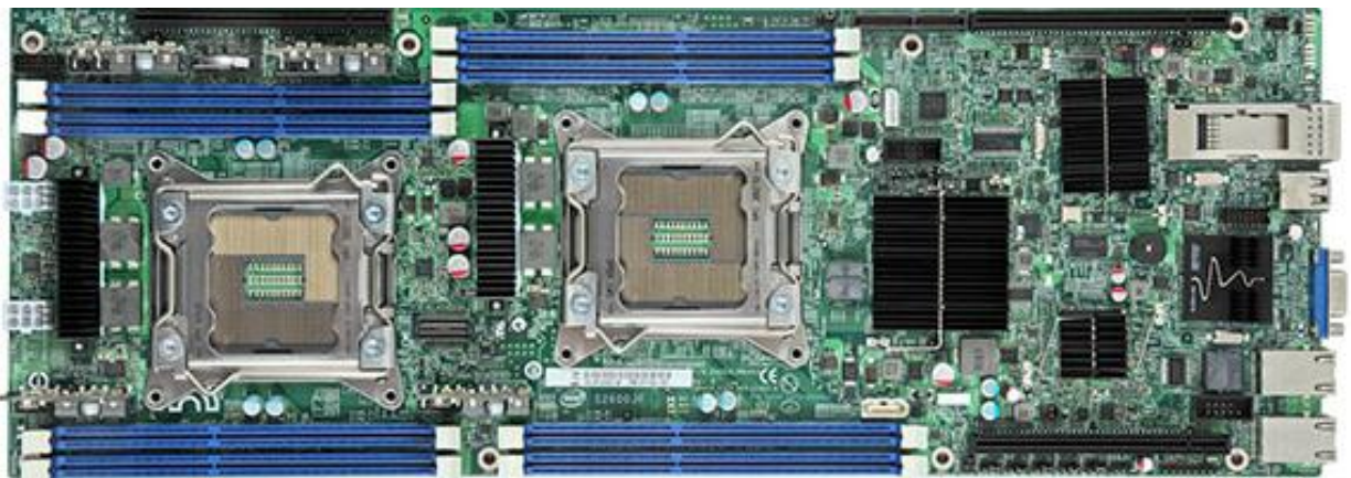
Figure 5-2 Intel S2600 series motherboard real item top view photo
