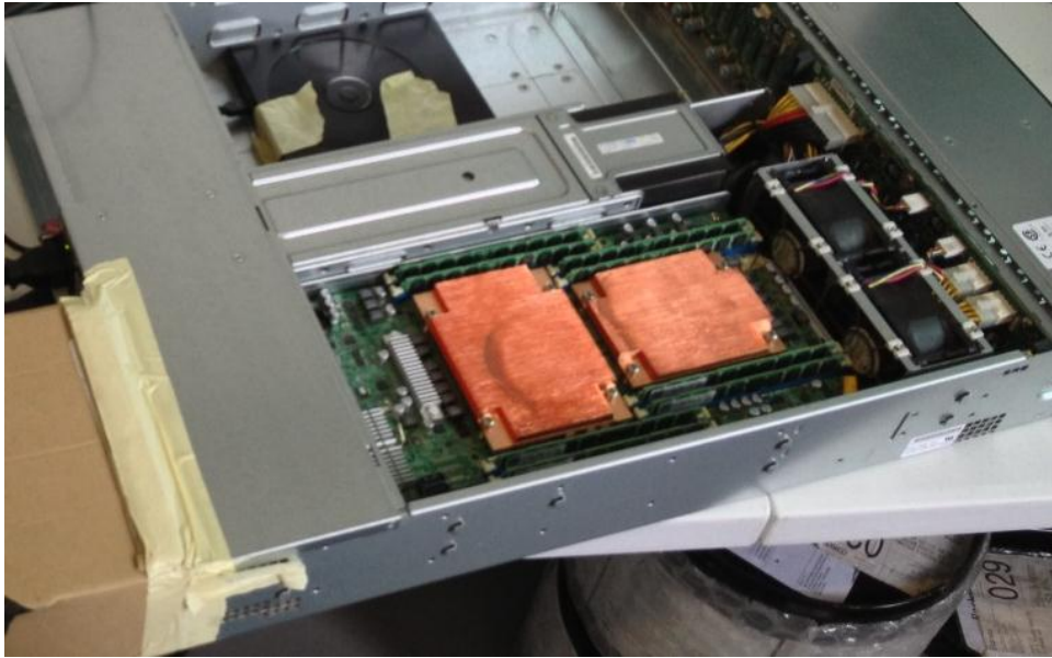
Figure 6-7 The computer node (node 107) in an air-cooled configuration ready for experiment.
