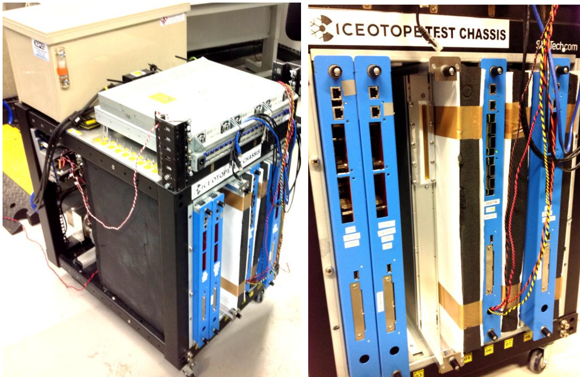
Figure 5-25 Photo of the thermal test unit in the Iceotope company lab
