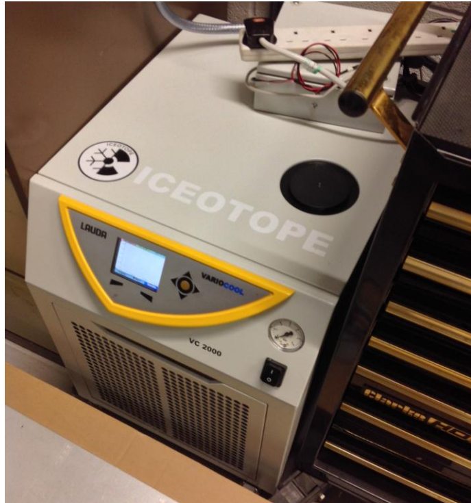
Figure 5-26 Heat rejection unit in the lab which can provide constant water temperature
