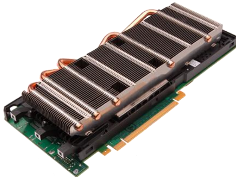
Figure 2-18 Standard nVIDIA M2070 GPU unit with passive heat sink and heat pipes (nVIDIA, 2011)
