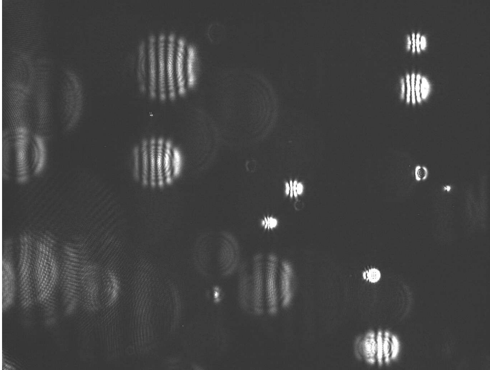
Figure A-0-1 Interference fringes from olive oil droplets and a 10x microscope objective
