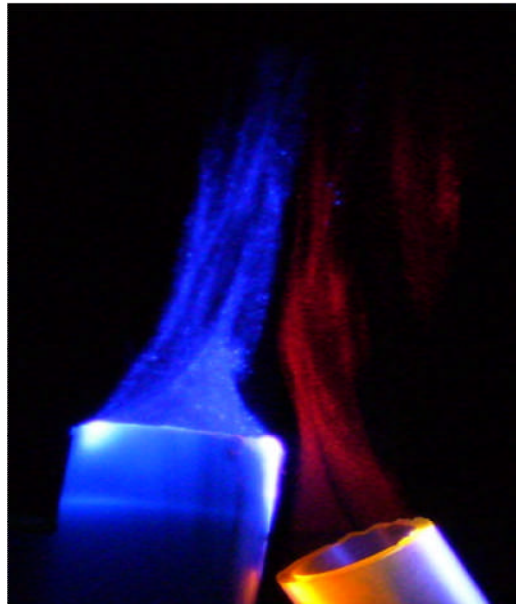
Figure 5-1 Bis-MSB (left) and DCM (right) tracers excited by a 355 nm laser light sheet.
