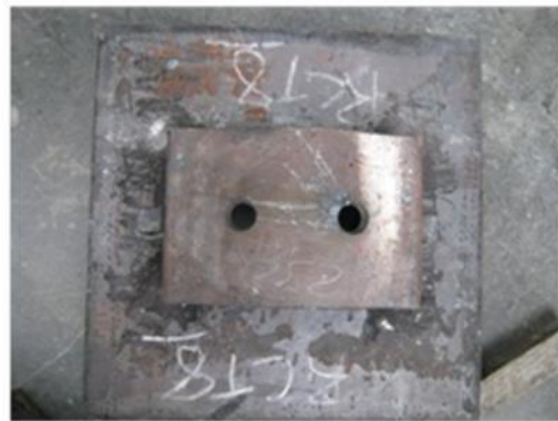
Figure 21: Straight yield line plastic hinge mechanism (RCT 8) (RFCS, 2012a).
