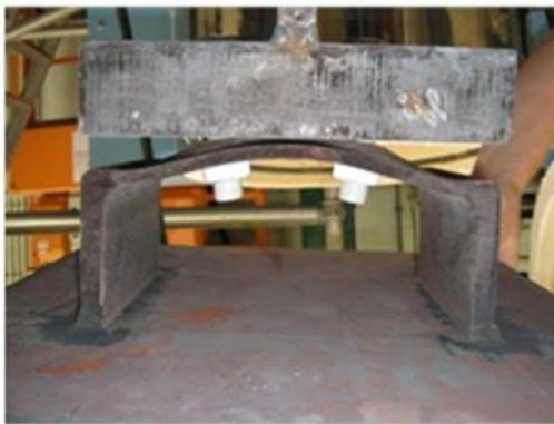
Figure 21: Straight yield line plastic hinge mechanism (RCT 8) (RFCS, 2012a).
