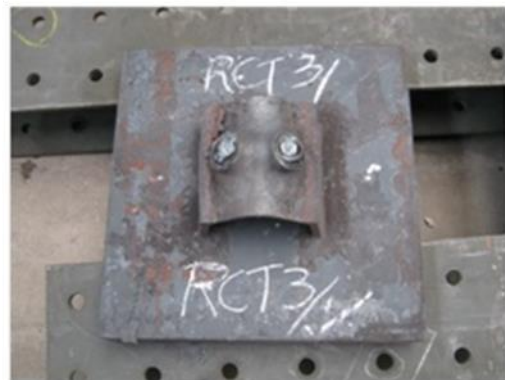
Figure 22: Circular yield line pattern and plastic hinge mechanism (RCT3) (RFCS, 2012a).
