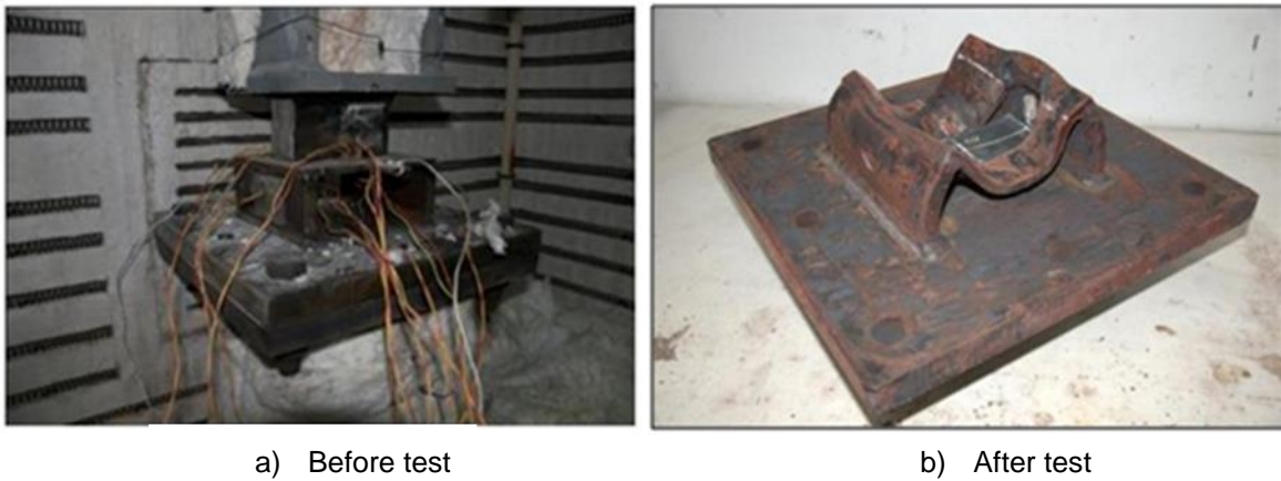
Figure 67: Test 13: welded reverse channel 202x200x10; compressive load; 750°C [University of Coimbra].
