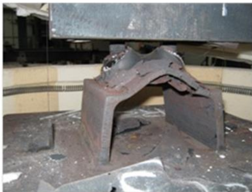
Figure 22: Circular yield line pattern and plastic hinge mechanism (RCT3) (RFCS, 2012a).
