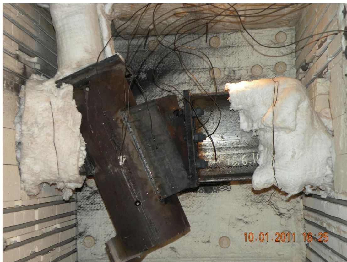
Figure 170: CCFT-RC200_550_55_10-01-2011 side view after test
