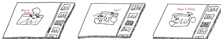
Figure 5.8: Rotate a window using one or two hands. (left) Press with two fingers from one hand and move both fingers to rotate. (middle) Press with two hands and drag one hand to rotate window asymmetrically. (right) Press with two hands and drag both hands to rotate window symmetrically.
