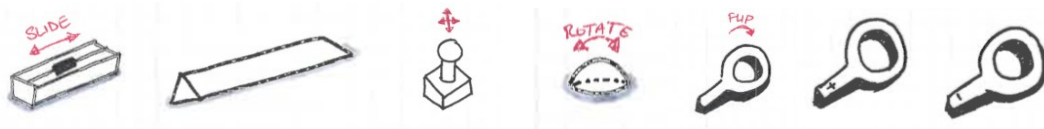
(a) Objects to pan plots and scroll tables. (b) Objects to zoom a plot. (left) A dial (left) A slider to manipulate and scroll a object to rotate and zoom. (middle) One table or pan plot. (middle) An abstract magnifier object to zoom. (right) Two object to brush window to pan or scroll. magnifier objects, one to zoom in and the (right) A joystick to pan a plot. other to zoom out.
