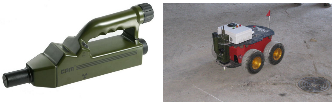
Figure 5.10: Left: The Chemical Agent Monitor (CAM) developed by Smith's Detection (formerly Graseby Dynamics) [SmithsDetection, 2010b]. Size: 350 x 80 x 145mm. Weight: 1.9kg (including standard battery). Power Source: Single 6V battery, rechargeable battery, or 4 x D-cell batteries with training adaptor. Right: The CAM mounted on a Pioneer Robot [Mobile-Robots, 2010].
