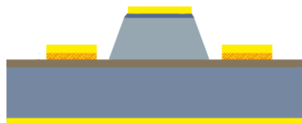
Figure 2.12: Schematic of the QCL after substrate thinning and metallization. The thickness of the substrate is reduced from \sim 500 \mu\text{m} to \sim 200 \mu\text{m} .
