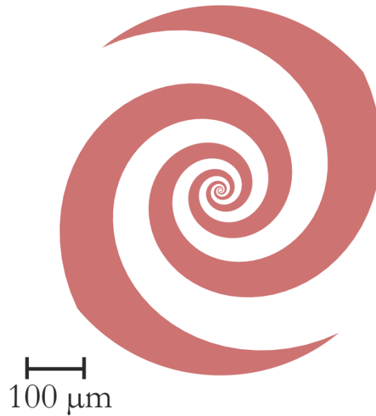
Figure 4.8: Schematic of the 3-turn self-complementary log-spiral antenna used with an active area of 11.3 \mu\text{m} \times 11.3 \mu\text{m}
