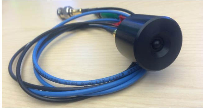
Figure 3.8: Photographic image of the fibre coupled commercial photomixer-emitter, TOPTICA.
