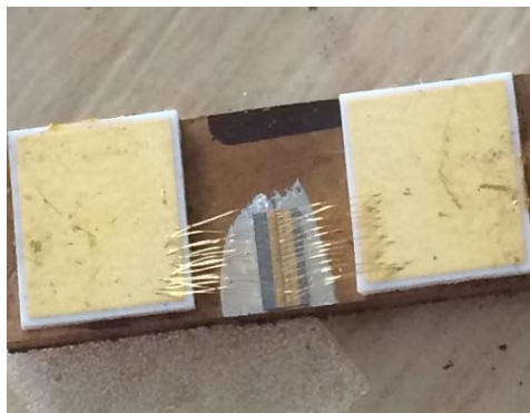
Figure 2.13: Photographic image of the QCL mounted on the copper block and wire bonded to contact pads.
