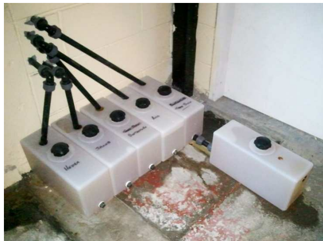
Figure 7.10 Water tanks to collect the excess water released from each test bed system. The trough system discharged more water than the others, thus it had double tanks (2012)
