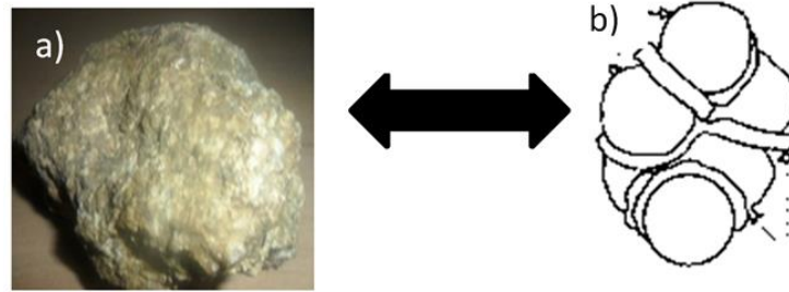
Figure 2.11 Conceptual illustration of the present research: a) macro structure of natural sandstone. b) Numerical simulation of particles and inter-particle cementing material representing the natural sandstone.
