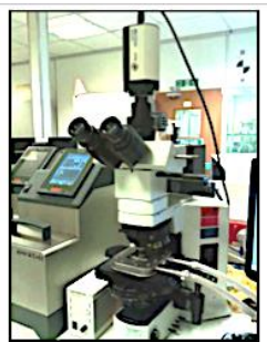
Figure 4-6 Upright Olympus BX15 microscopy equipped with transmitted light with capabilities to measure length and observe morphology of crystal
