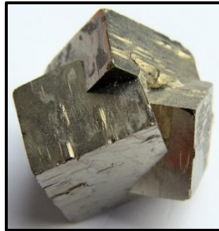
Figure 2-9 Twinning in Pyrite crystal showing clear mirroring of parent structure (Figure from [37])
