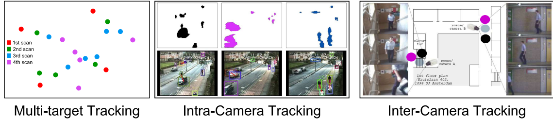
Figure 2.19: The three different data association problems are shown. In each problem, the detections are partitioned into a previously unknown number of targets or considered false detections. Intra-camera diagram taken from [149] and inter-camera diagram from [150]
