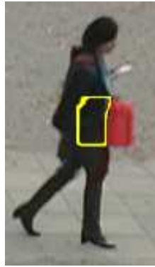
Figure 6.9: The red-coloured region signifies the pixels added to the carried object's colour histogram, while the yellow-bounded region signifies the neighbouring region's pixels.
