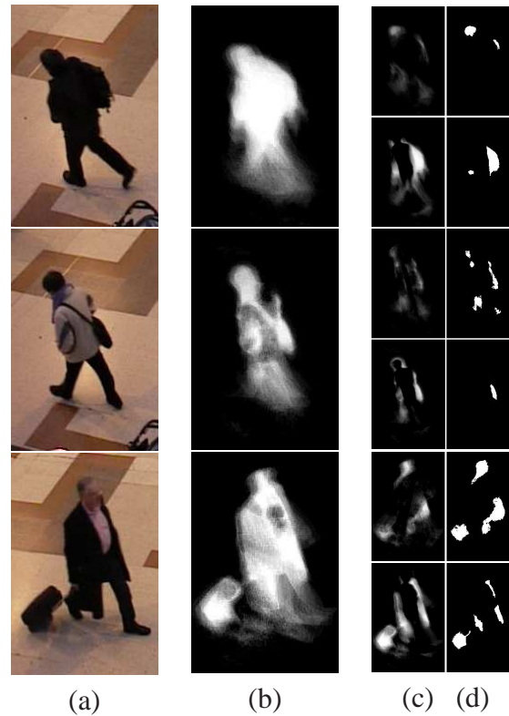
Figure 7.12: Three examples (a), along with their temporal templates (b) are assessed using both techniques. The asymmetric regions (c-top) thresholded (d-top) and the protruding regions (c-bottom) thresholded (d-bottom) show some examples of how template matching retrieves better estimate of the carried objects.
