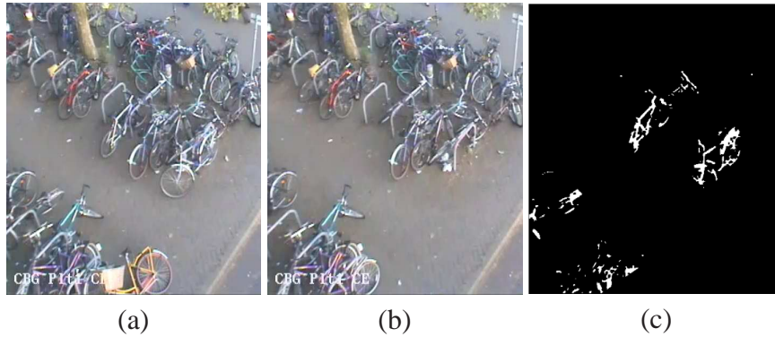
Figure 5.4: Before (a) and after (b) reference images, revealing changed pixels (c) that signify 3 picked bicycles and one dropped bicycle.
