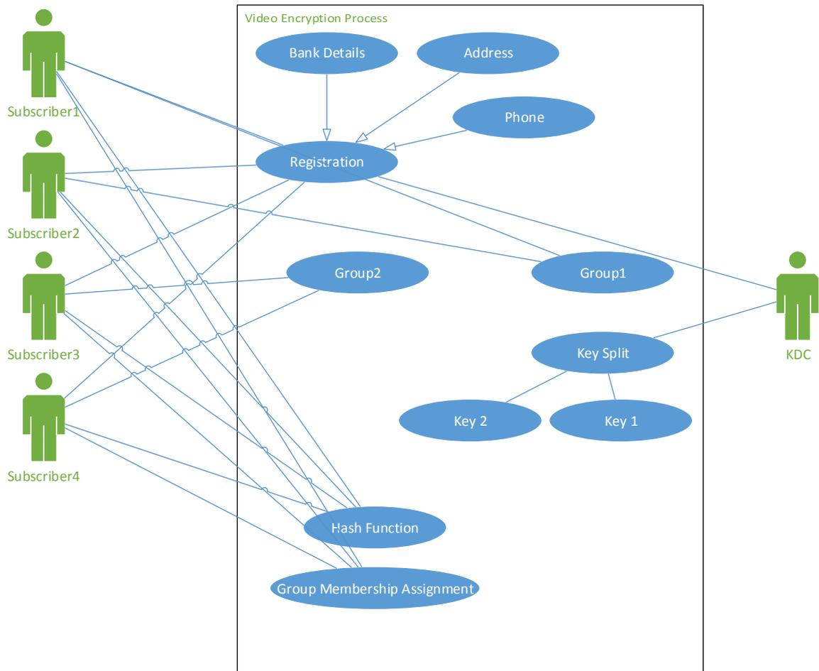
**Figure 16: Use case diagram for the video encryption using secret sharing**
