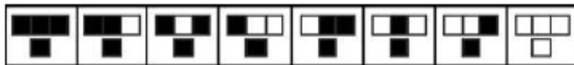
Figure 4.18. Graphical depiction of a CA state transformation function. A shaded square has a state 1, and unshaded state 0 (Frans et al., 2007).
