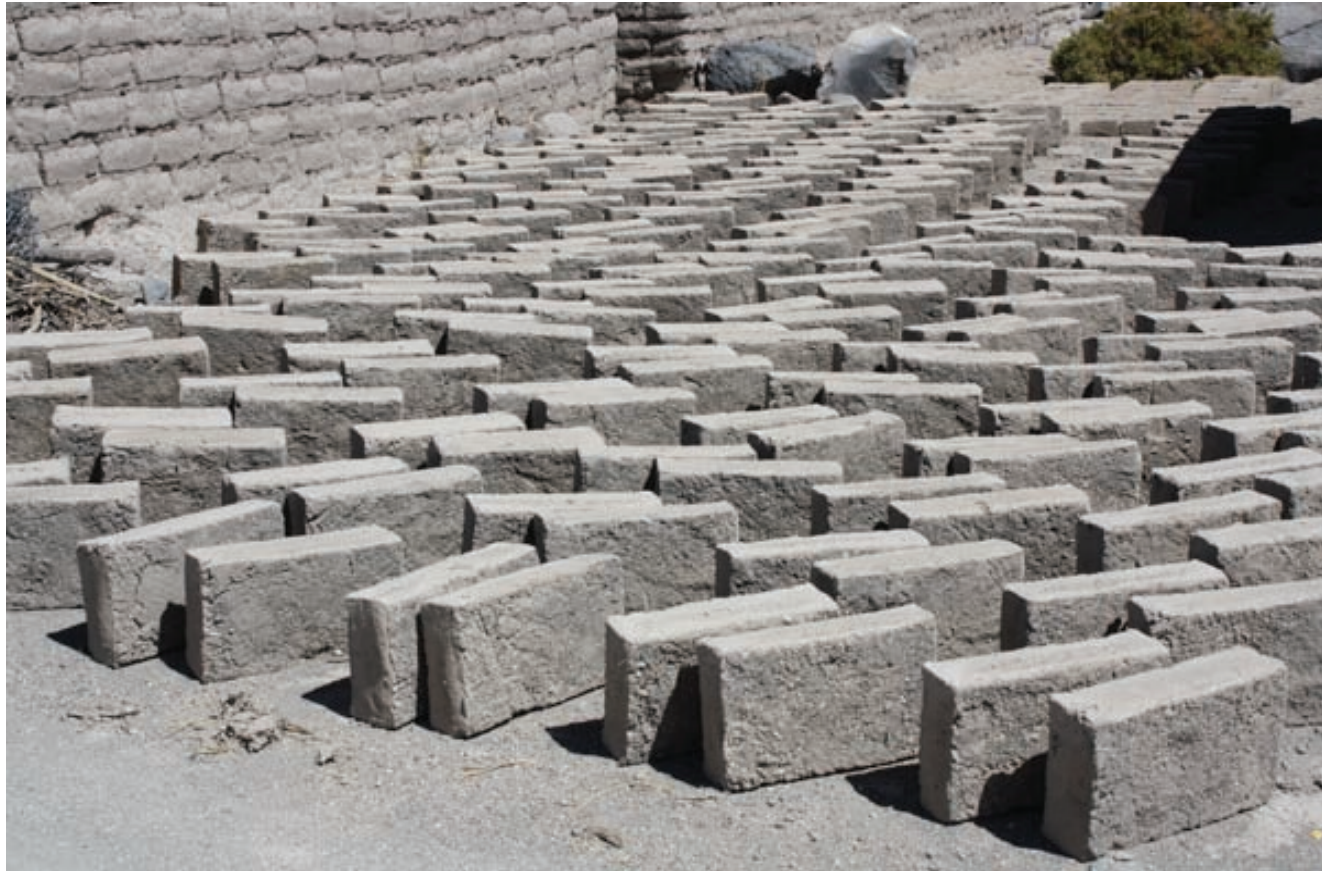
Fig. 4.28 Adobe bricks drying in the sun.
