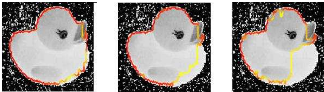
Figure 6.19: Segmentation results of region growing with different threshold value on a real world image [254]: From the left Q_3 = 0.81, 0.70, 0.49 . Colours of the boundary pixels correspond to \xi_3 .
