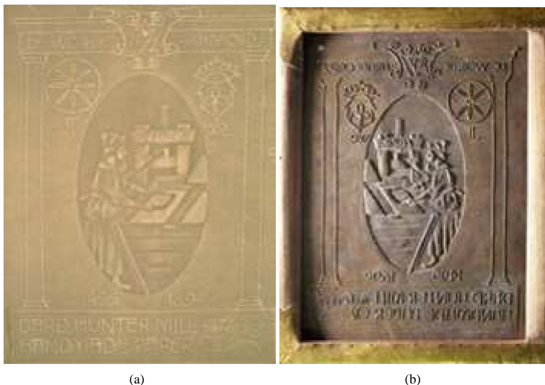
Figure 2.3: (a) Light and shade watermark, (b) Mould used to produce this watermark. With permission from Cindy Bowden [104]
