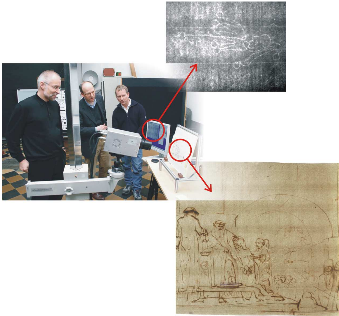
Figure 2.33: Thermography setup, with a watermark image result. With permission from Peter Meinschmidt [50]
