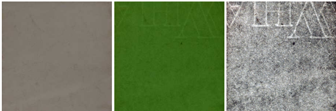
Figure 5.5: Scanned, backlit and differenced images (left to right) – the watermark is clearly revealed. The difference has been contrast stretched for display. This image is a part of the full illustrated paper shown in Figure B.1 in Appendix B. This document is taken from the works of Henry Litolff [14], digitised with permission from the Special Collections at the Brotherton Library of the University of Leeds [123].
