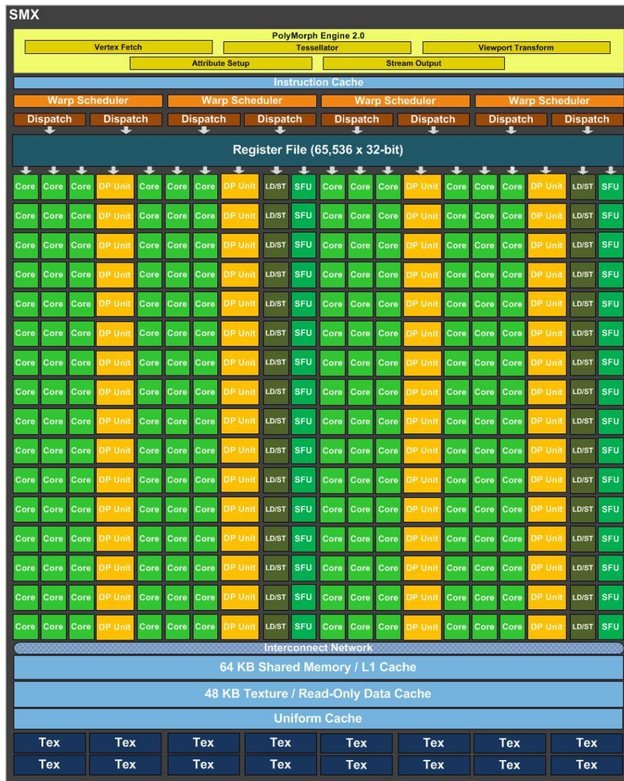
Figure 94: Architecture of one Streaming Multiprocessors for the Tesla K40 (GK110B) NVIDIA GPU. Source: NVIDIA.
