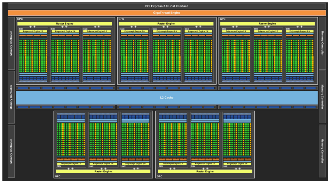
Figure 95: Architecture of the Tesla K40 (GK110B) Nvidia GPU. Source: Nvidia. (see zoom on figure 94)
