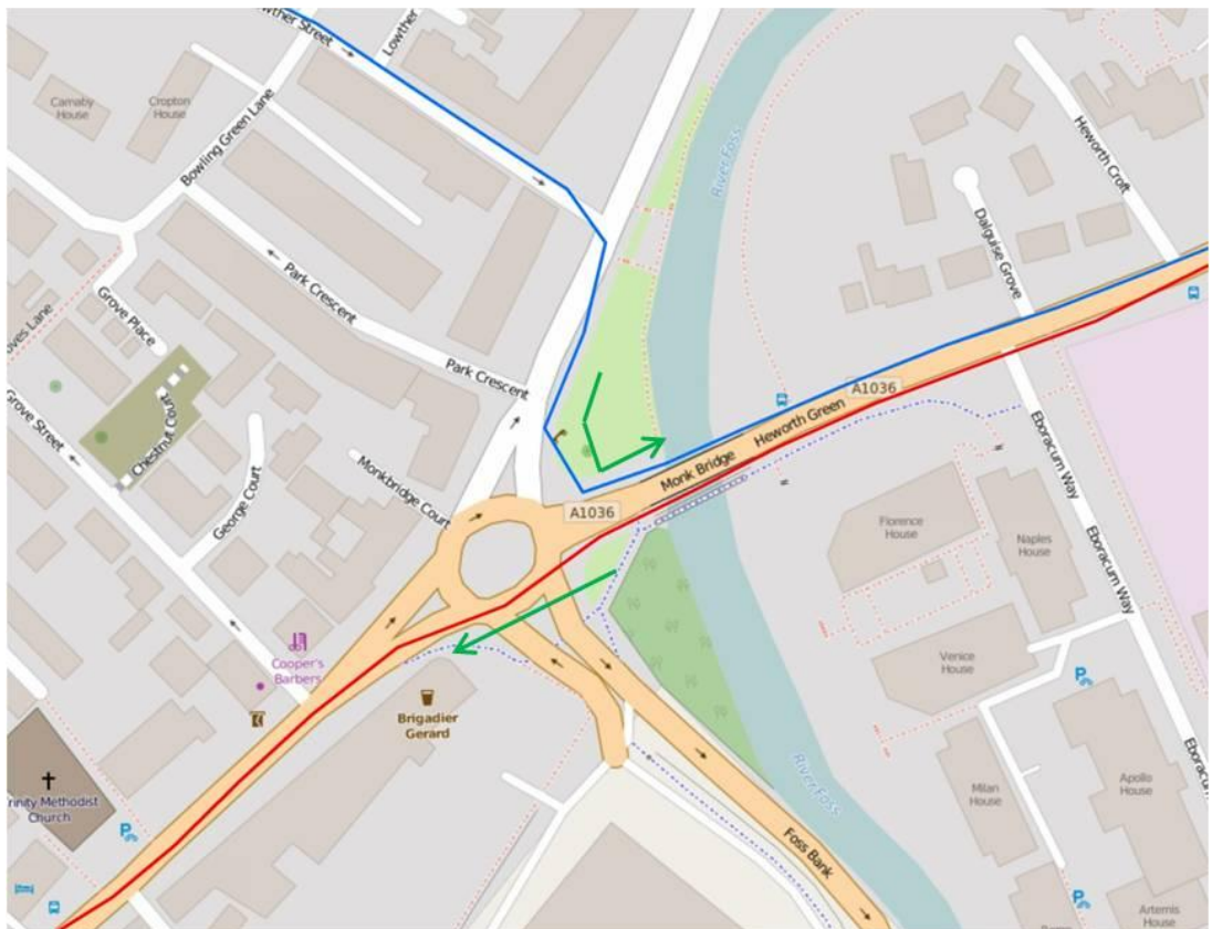
Figure 5.5 Example of Detouring by Junction (Y9)
