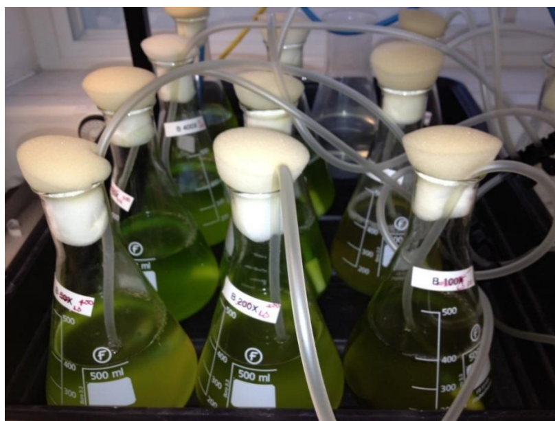
Figure 8-13: C.vulgaris growing in diluted SCWG aqueous products from microalgae, L.digitata and sewage sludge
