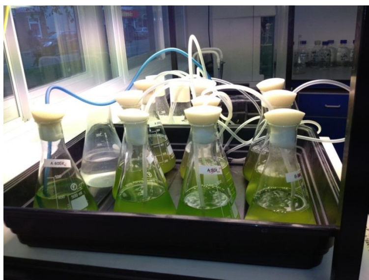
Figure 3-8: 500mL bioreactors showing growth of C. vulgaris in various dilutions of the HTG process water from various feedstocks
