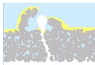
Figure 10. A schematic representation of e-beam shadowing.
