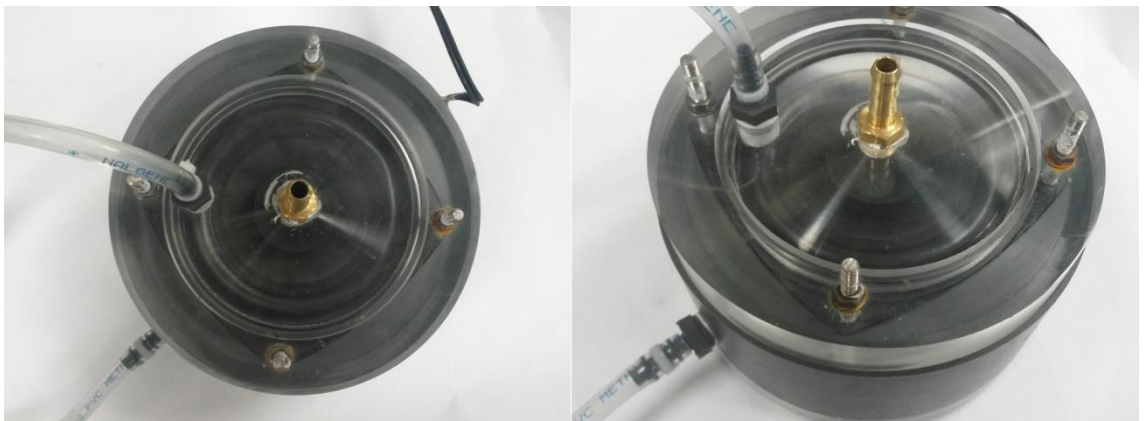
Figure 5-7 Visaton FR10 8Ω speaker was encased in a PVC and Perspex box as shown. 6 mm and 8 mm hose barbs were added to allow air flow in and out. Flow entered the top and bottom faces of the speaker and flow exited through the top (brass) fitting.
