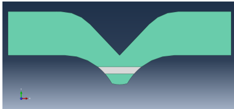
Figure 3.15 A hybrid_3 with horizontal energy absorbing strip below initiation point.
