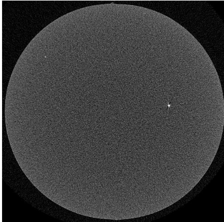
Figure 11 Display of a 2D image of a further processed O-ring_1. The image contains a visible void in the centre region of the image.
