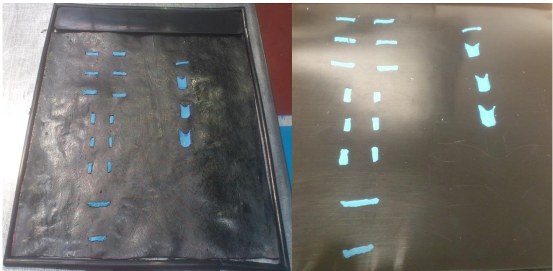
Figure 3.14 A hybrid tear sample test sheet before and after being cured for 12 minutes at 170 °C.
