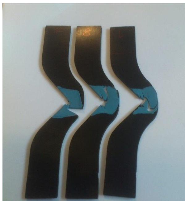
Figure 8.3 Failed specimens of hybrid 2 tearing strength sample (HNBR101 and LRCM888) cracks found it more difficult to propagate once they initiated in the LRCM888 layer.
