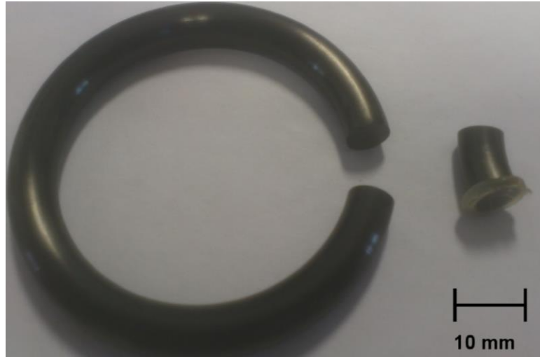
Figure 3.5 A sectioned O-ring specimen analysed using computerised tomography.
