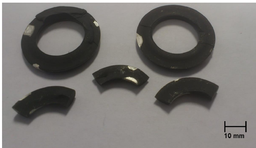
Figure 3.1 Fractured Fluorocarbon FKM type 3 O-ring specimens, the silver paint increases the specimen's conductivity.
