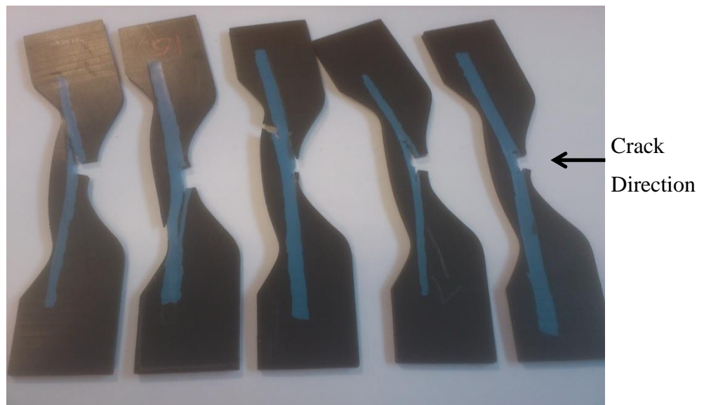
Figure 8.7 Display of fractured hybrid 1 fatigue samples with a second phase material located behind the crack initiation point.
