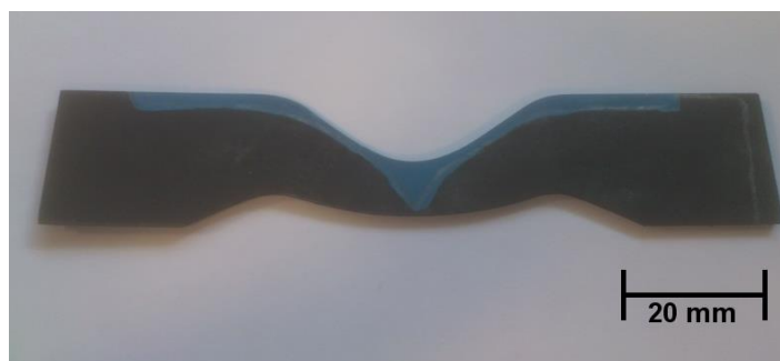
Figure 3.21 Hybrid fatigue sample 3 with a second phase material located in the region of high stress concentration.
