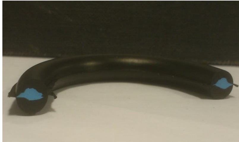
Figure 8.23 Hybrid_1 O-ring with a circular second phase material located in the centre region of the O-ring.
