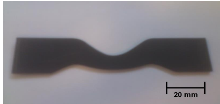
Figure 3.18 A control fatigue sample with no second phase material (HNBR101 only).
