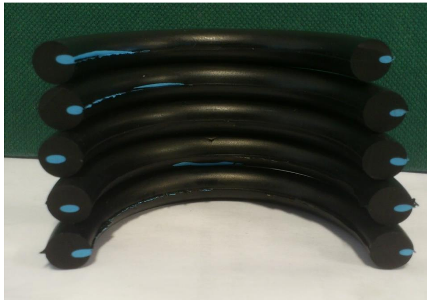
Figure 8.26 Hybrid _2 O-ring with a horizontal oval second phase material located in the centre region of the O-ring, manufactured using the pre-curing technique.
