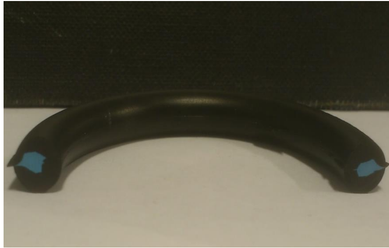
Figure 8.25 Hybrid _3 O-ring with a vertical oval second phase material located in the centre region of the O-ring.
