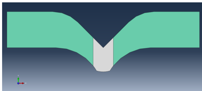
Figure 3.16 A hybrid_4 with energy absorbing layer located at the point of crack initiation.
