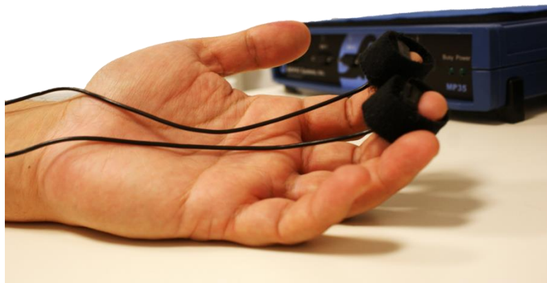
Figure 4.1 Electrodermal activity electrodes attached over the distal phalanx of the index and middle finger.
