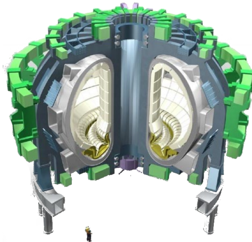
Fig. 1.5 The arrangement of toroidal (blue), poloidal (green) coils and divertor (yellow) within a Tokamak. Image source [48].
