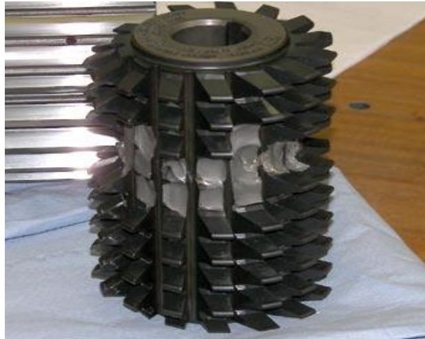
Figure 5.2 Breakage of hob cutter
