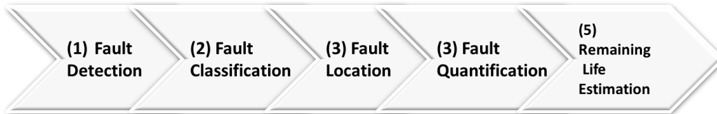
Figure 3.2 The stages of condition monitoring (adapted from [7])
