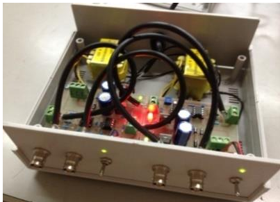
Figure 4.11 Two-channel signal amplifier
