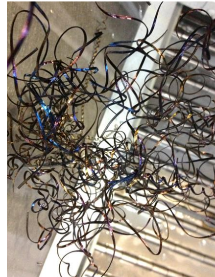
Figure 6.26 Chips removed from the workpiece in the failure wear state
