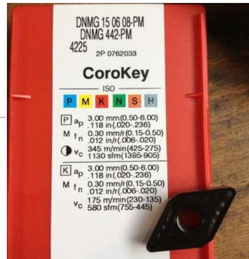
Figure 6.6 The product information of cutting insert used in this machining experiment
