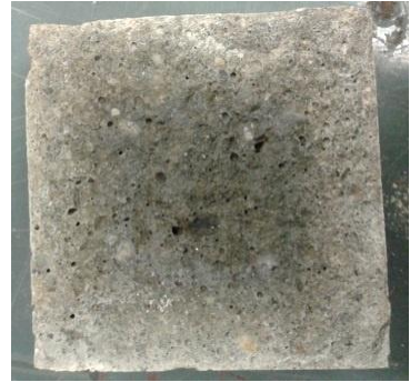
Plate 1: Pictures showing extent of chloride penetration into mortar samples exposed to a 3% NaCl solution at 20°C for 90 days
