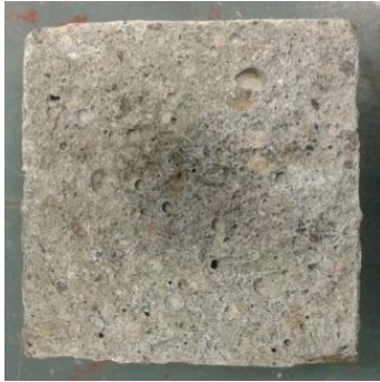
Plate 1: Pictures showing extent of chloride penetration into mortar samples exposed to a 3% NaCl solution at 20°C for 90 days
