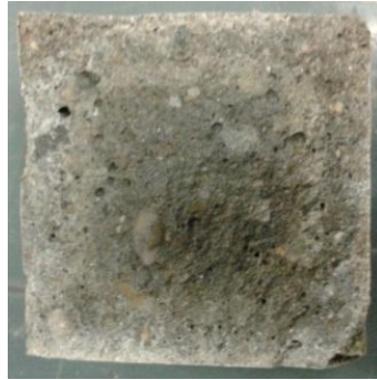
Plate 1: Pictures showing extent of chloride penetration into mortar samples exposed to a 3% NaCl solution at 20°C for 90 days
