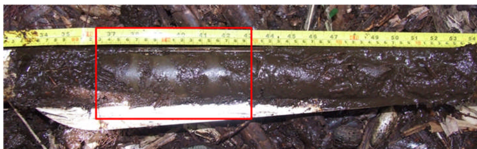
Figure 5.5. A section of the Ekolongouma 9 km core. The red box highlights points in the profile where mineral intrusions can be seen.
