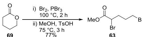
Figure 22: The synthesis of methyl 2,5-dibromovalerate 63 from \delta -valerolactone 69 via \text{PBr}_3 -mediated bromination.
