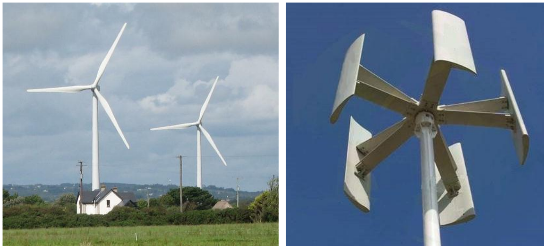
Figure 2. On-shore HAWTs (left) and a typical VAWT (right).
