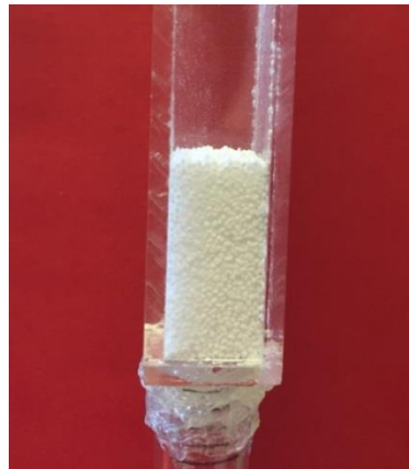
Figure 4-6. Sample preparation for XRT scan (using 3 g of 850 \mu\text{m} near-mesh burkeite particles)
