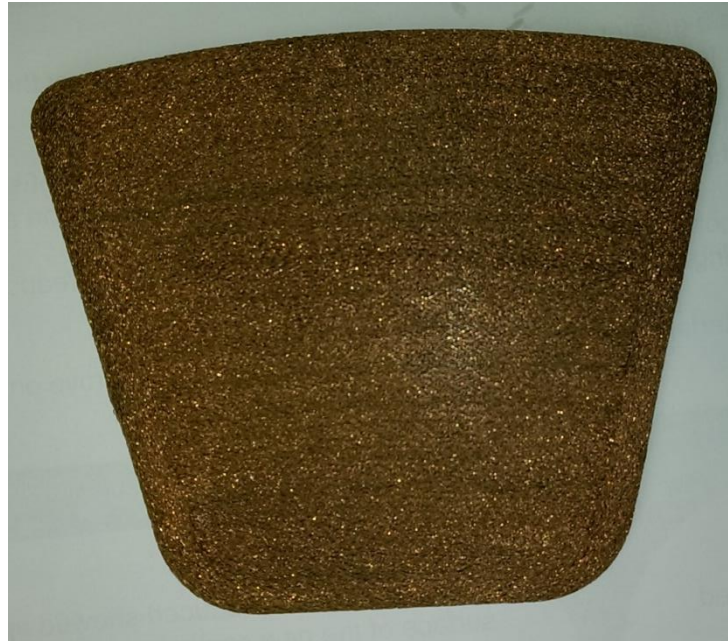
Figure 2.15 Copper mesh used to bond PTFE to steel backing material
