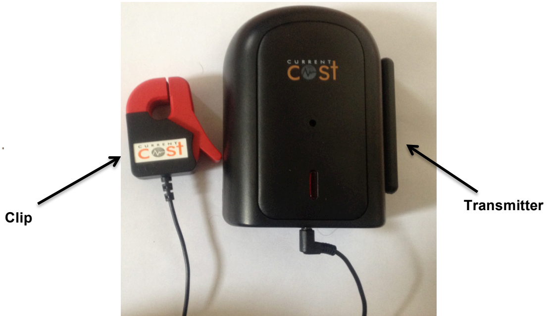
Figure 3.1: An example of the mains sensor
