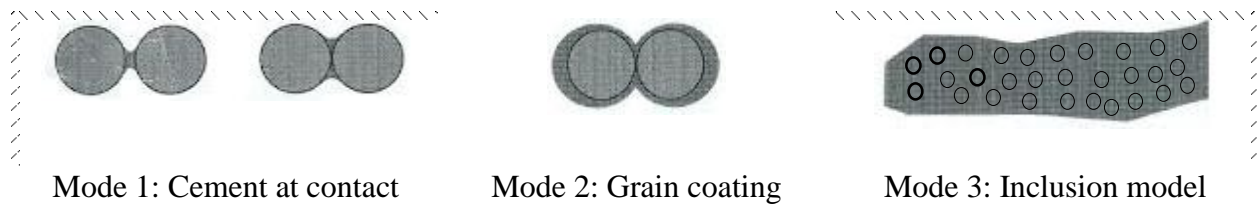
Fig. 8.3 Relative effects of three (3) common modes of ice contents on lunar soil strength
