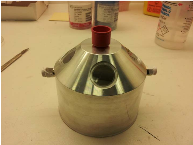
Figure 3.8: The cover to control atmosphere around a spin-coating stage.
