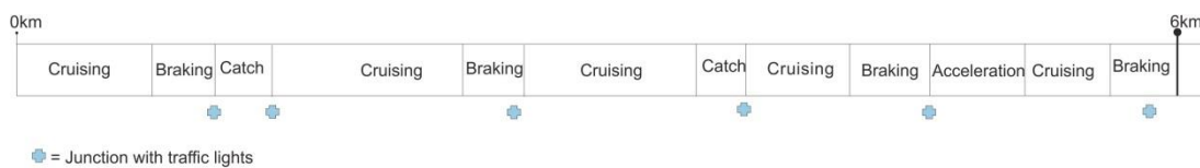
Figure 14: Example of an urban section with acceleration, braking and cruising scenarios
