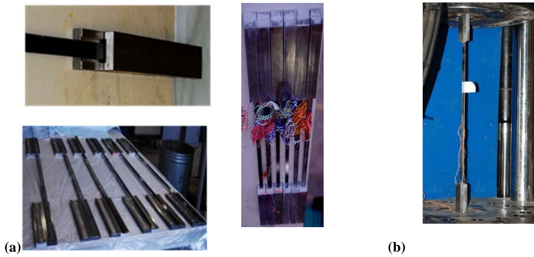
Fig. B - 4: Preparation of tensile tests and FRPs (a) specimen preparation (b) test set up
