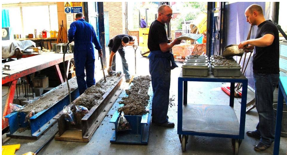
Fig. B - 17: Concrete casting and curing
