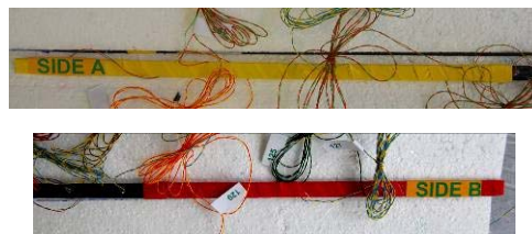
Fig. B - 18: Strain gauges bonded on strips before strengthening
