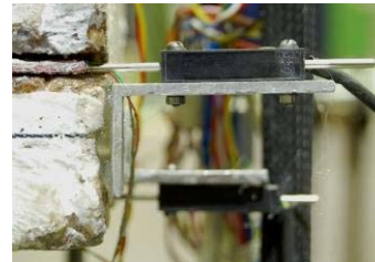
Fig. B - 15: Details of set up of LVDTs at the LVDT group C
