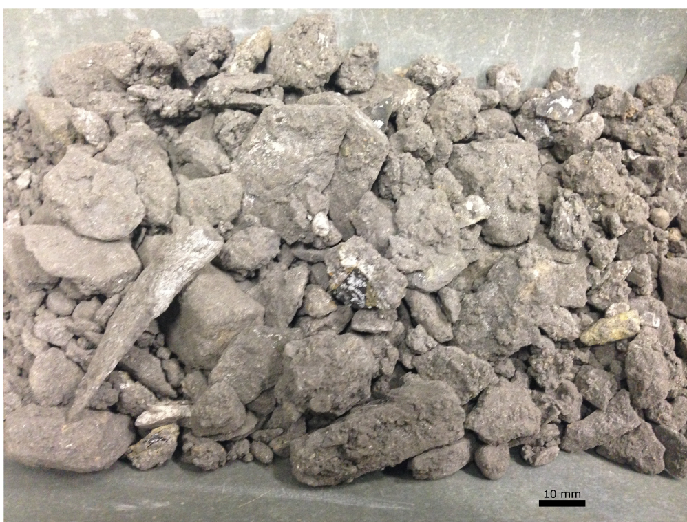
Figure 7.13: Mudrock fill material used in the laboratory testing in its dry state as used for the Comparison Testing
