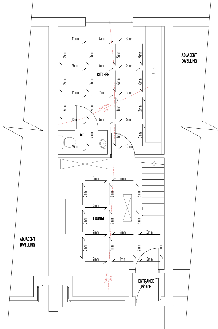
Figure 7.14: Floor level survey for the property from which the samples were taken (used with permission of Aidan O’Connell Associates). All marked lines showing changes in floor level are 1 metre in length.
