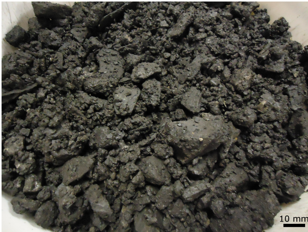
Figure 7.3: Mudrock fill material used in the laboratory testing in its damp state.
