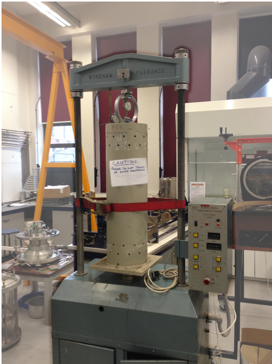
Figure 8.21: Placement of swell test 10 within the triaxial frame.
