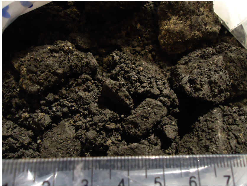
Figure 6.12: Material taken from the pit in which the sensors were installed, shown at its natural moisture content.
