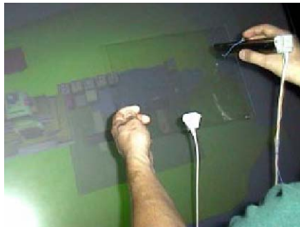
Figure 5-6 The pen-and-pad interface on the Virtual Table in [Schmalstieg & Encarnacao 1998]
