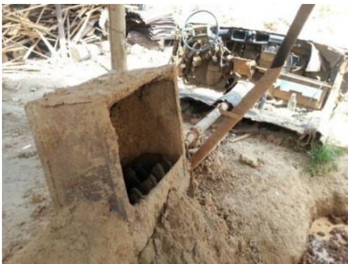
Snapshot 3 Mixer technology, reclaimed automobiles’ engines
